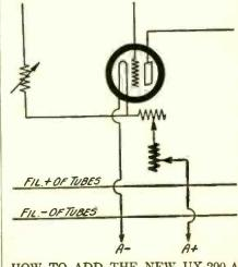
HOW TO ADD THE NEW UX-200-A DETECTOR TUBE
