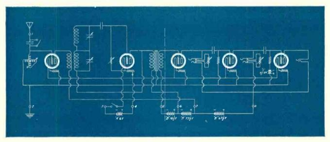
THE CIRCUIT DIAGRAM OF THE CONVERTED RECEIVER FIGURE 4: The circuit to the left of the broken line is identical with that of the LC-26; to the right of this line it is similar to that of the Four-circuit Tuner.
