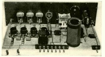
A REAR VIEW OF THE CONVERTED FOUR-CIRCUIT TUNER RECEIVER
