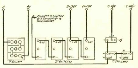
THE HOOK-UP FOR THE BATTERIES FIGURE 3: This drawing gives the correct battery circuit and the voltages for all of the batteries that are used to operate the new unit. SEPTEMBER, 1926
