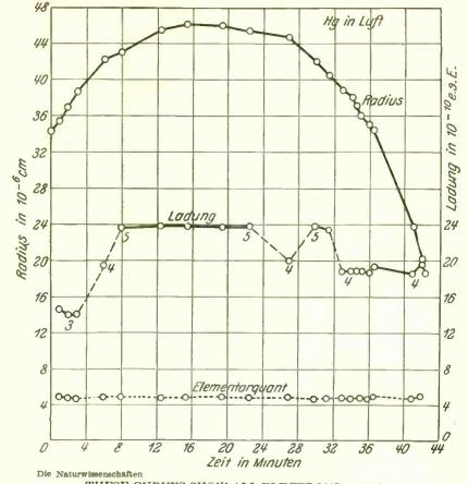
THESE CURVES SHOW ALL ELECTRONS ALIKE The upper curve shows the size of the floating mercury droplet; first increasing, then decreasing. The mildle curve shows the electric charge on this droplet, the figures indicating the number of electrons on the droplet from time to time. The bottom curve shows these figures reduced to the basis of one electron. The straightness of this bottom curve proves that all the electronic charges were equal.
