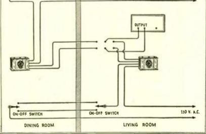
HOW THE CONNECTIONS ARE MADE These two drawings show the wiring arrangement for the dual operation of the set and loudspeaker installations on both the first and second floors of the "radio house."
