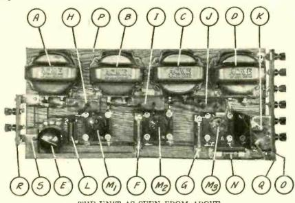
THE UNIT AS SEEN FROM ABOVE FIGURE 2: The general layout of the apparatus as it is mounted on the baseboard. The input binding posts are located at the left and the output jack is located at the right on the same strip as the "A'," "B" and "C" battery terminals.
