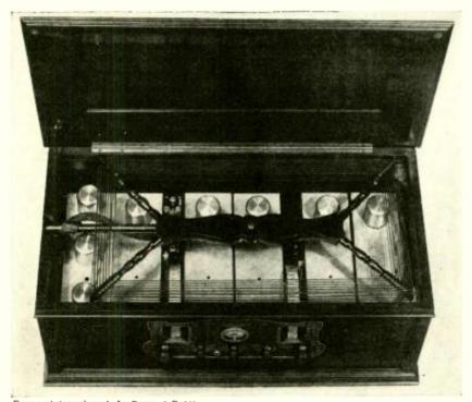
From a photograph made for POPULAR BADIO HOW THE LOOP FITS INTO THE CABINET FIGURE 3: This model differs from that shown in Figure 2 only in the smaller cabinet that is used. Note the shields that cover the apparatus.
