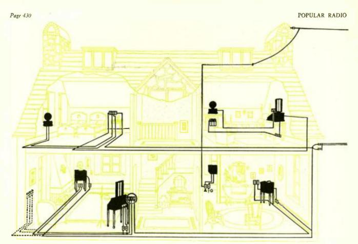
AN ACTUAL HOME THAT IS WIRED FOR WIRELESS Every room of this "radio house," (which is located on Staten Island, N. Y.) is served by radio, either in the shape of a complete receiver and loudspeaker installation or an extension loudspeaker unit with its own power amplifier. The wiring is as complete and as inconspicuous as the ordinary electric light wiring.
