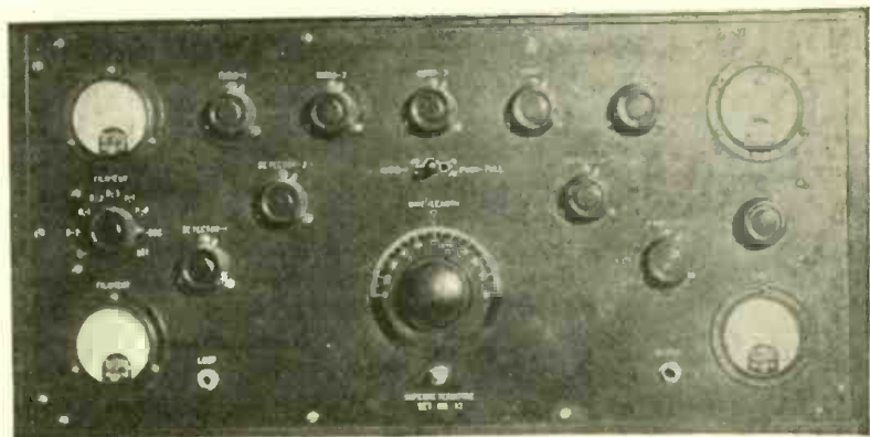
A SINGLE-CONTROL SUPERHETERODYNE WITH FOUR METERS INSTALLED
