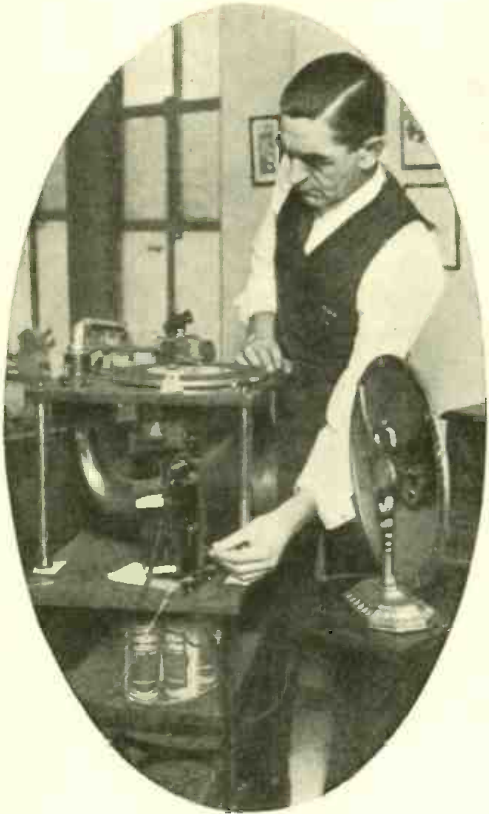
Let flippant announcers and off-key singers beware, for their broadcasting sins may be recorded for future generations of radio fans by means of this radio recording apparatus, invented by Francis R. Hoyt. It operates much as the machines which make records for your phonograph.
