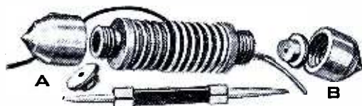
Assembly of the Leak and Condenser.
