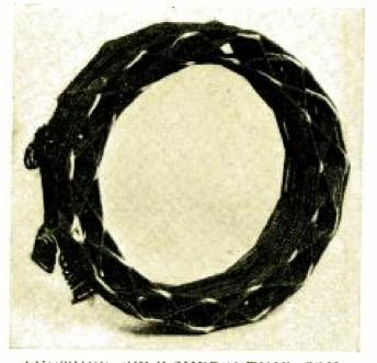
ANOTHER SELF-SUPPORTING COIL FIGURE 6: .1 special form of multi-layer coil, in which the losses were found to be excessive as compared to the straight singlelayer solenoid type of winding.
