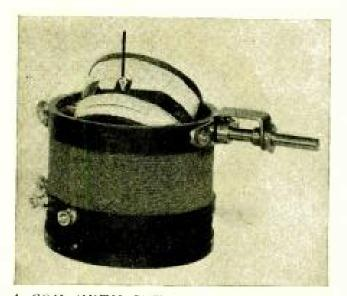
A COIL WITH CUT-AWAY INSULATOR FIGURE 3: A cut-away coil wound with multistrand wire that has been found to be almost but not quite as efficient as the straight solenoid type.
