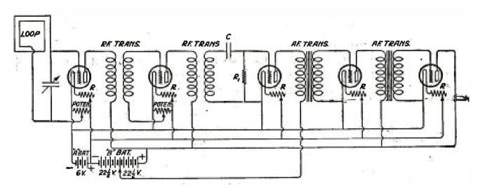
TWO STAGES OF RADIO, DETECTOR, AND TWO STAGES OF AUDIO-FREQUENCY AMPLIFICATION
