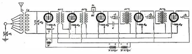
TWO STAGES OF TRANSFORMER-COUPLED RADIO-FREQUENCY AMPLI-FICATION WITH VACUUM-TUBE DETECTOR AND TWO STAGES OF AUDIO-FREQUENCY AMPLIFICATION
