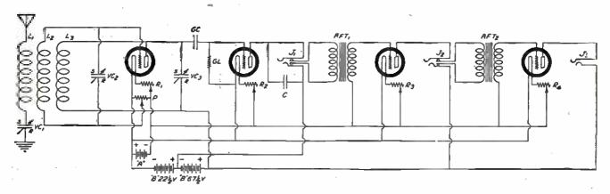
ONE STAGE OF TUNED-RADIO-FREQUENCY AMPLIFICATION, VACUE TUBE DETECTOR AND TWO STAGES OF AUDIO-FREQUENCY AMPLIFICATION EMPLOYING HONEYCOMB COILS FOR TUNING VACUUM
