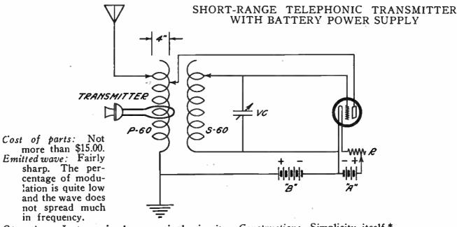
Operation: Just as simple as a single-circuit receiving set. The UV-201-a tube may be used with about 100 volts of "B" battery for the plate supply.
