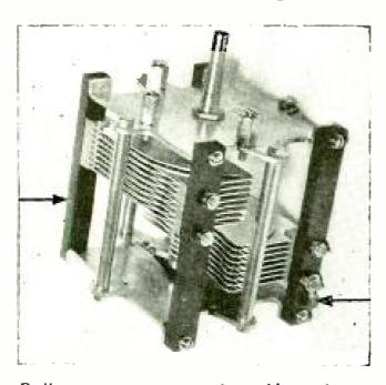
Radion separators are used on this condenser with soldering lugs for connections.
