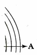
"A" is a stray field or wave, traveling toward the coil. Due to the winding all induced currents oppose each other so no current can flow. Hence no pick-up.
