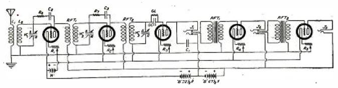
THE PLIODYNE PRINCIPLE INCORPORATED INTO A RADIO-FREQUENCY CIRCUIT WITH VACUUM-TUBE DETECTOR AND TWO-STAGE AUDIO-FREQUENCY AMPLIFIER
