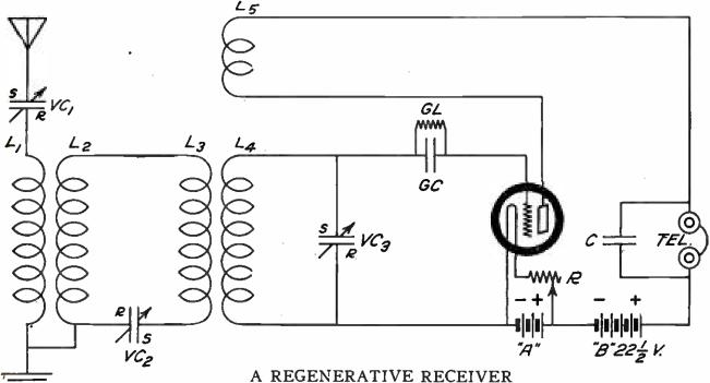
WITH AN INTERMEDIATE CIRCUIT TO REDUCE RADIATION
