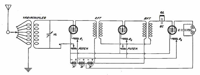
TRANSFORMER-COUPLED RADIO-FREQUENCY CIRCUIT WITH VACUUM-TUBE DETECTOR
