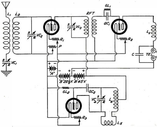
ONE STAGE OF TUNED-RADIO-FREQUENCY, VACUUM-TUBE DETECTOR, WITH SEPARATE HETERODYNE FOR CW RECEPTION
