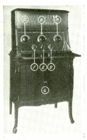
A, B and C are the tuning dials. D, E and F are the rheostats and volume control. G is the container for the batteries.
