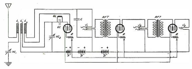
TRIPLE-COIL HONEYCOMB REGENERATIVE RECEIVER WITH TWO STAGES OF AUDIO-FREQUENCY AMPLIFICATION
