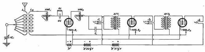
TWIN-VARIOMETER, VARIOCOUPLER REGENERATIVE CIRCUIT WITH TWO STAGES OF AUDIO-FREQUENCY AMPLIFICATION
