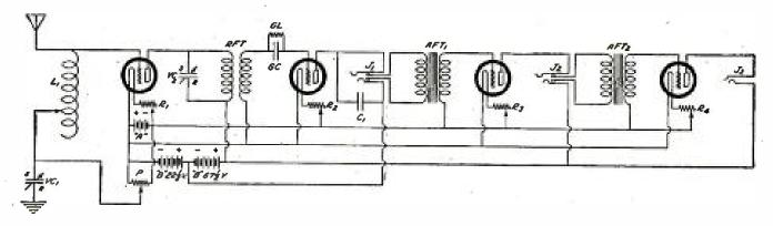
SINGLE-STAGE RADIO-FREQUENCY AMPLIFIER WITH TUNED-PLATE CIR-CUIT, DETECTOR, AND TWO-STAGE AUDIO-FREQUENCY AMPLIFIER
