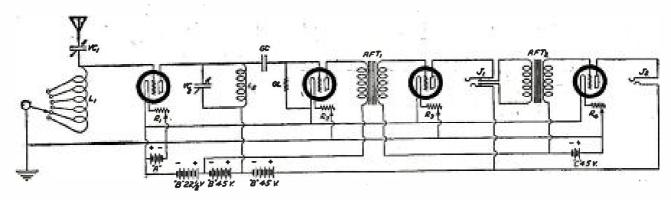
ONE STAGE OF TUNED-RADIO-FREQUENCY, DETECTOR AND TWO STAGES OF AUDIO-FREQUENCY AMPLIFICATION
