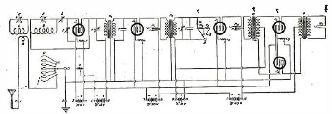
THE FOUR-CIRCUIT TUNER WITH TWO STAGES OF STRAIGHT TRANS-FORMER-COUPLED AMPLIFICATION, AND ONE STAGE OF PUSH-PULL AMPLIFICATION
