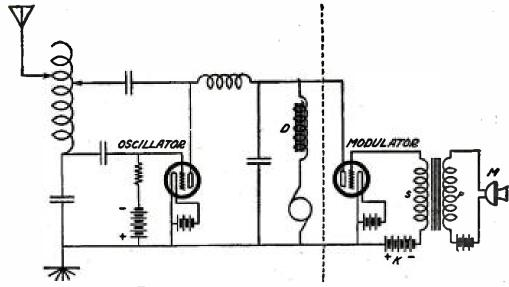
THE COLPITTS CIRCUIT WITH HEISING MODULATION
