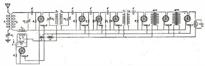
A RESISTANCE-COUPLED SUPERHETERODYNE WITH TWO STAGES OF AUDIO-FREQUENCY AMPLIFICATION
