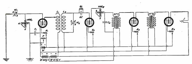
STAGE OF TUNED-RADIO-FREQUENCY AMPLIFICATION, WITH A VACUUM-TUBE DETECTOR AND TWO STAGES OF AUDIO-FREQUENCY AMPLIFICATION
