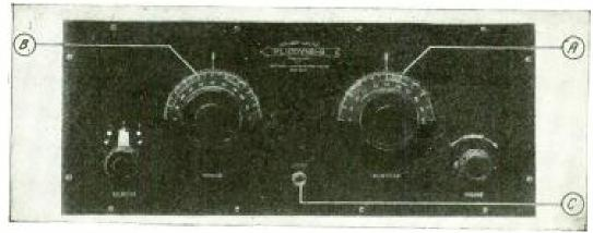
A and B are the tuning dials. C is the loudspeaker jack.
