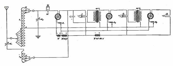
THE REINARTZ CIRCUIT, WITH TWO STAGES OF AUDIO AMPLIFICATION
