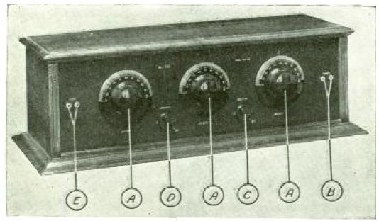
A are the three tuning dials. B are the plugs for the phones. C and D are the rheostats and E are the loudspeaker jacks.
