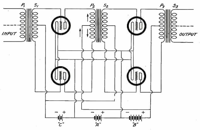
TWO STAGES OF PUSH-AND-PULL AMPLIFICATION.
