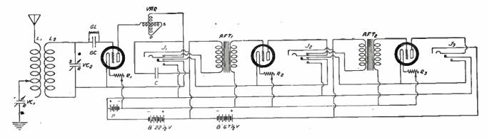
REGENERATIVE RECEIVER WITH TWO STAGES OF AUDIO-FREQUENCY AMPLIFICATION, EQUIPPED WITH AUTOMATIC FILAMENT-LIGHTING JACKS
