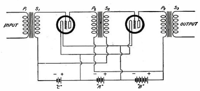
TWO-STAGE, TRANSFORMER-COUPLED, POWER AMPLIFIER FOR USE WITH 5-WATT TUBES
