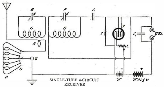
Cost of parts: Not more than \$24.00. Selectivity: Excellent. Operation: Simple. The condenser C1 should be of the correct value to put the set into stable condition and then the condenser E is adjusted so that the circuit is just on the highly regenerative point. All tuning is then accomplished with the condenser F and the antenna switch Q.
