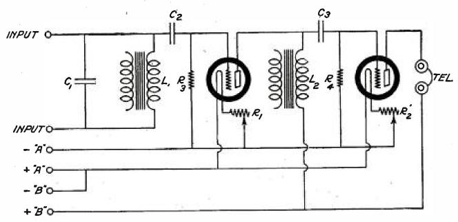
TWO-STAGE, IMPEDANCE-COUPLED AMPLIFIER MADE FROM FORD SPARK COILS
