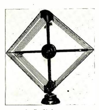
A collapsible loop antenna.
