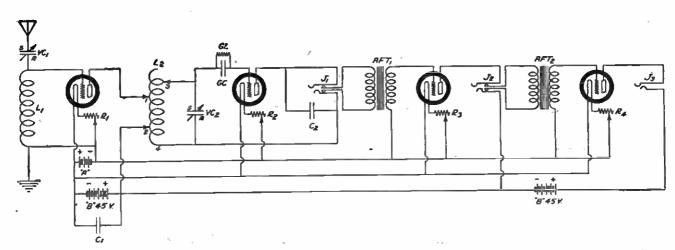
ABELE CIRCUIT COMPRISING ONE STAGE OF TUNED-RADIO-FREQUENCY AMPLIFICATION, VACUUM-TUBE DETECTOR AND TWO STAGES OF AUDIO-FREQUENCY AMPLIFICATION
