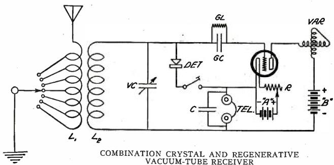
Cost of parts: Not more than \$27.00. Selectivity: Good (with crystal). Excellent (with vacuum tube). Operation: Simple.
