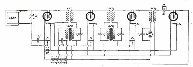
FOUR-TUBE REFLEX WITH THREE STAGES OF RADIO-FREQUENCY AMPLI-FICATION, VACUUM-TUBE DETECTOR AND TWO STAGES OF AUDIO-FREQUENCY AMPLIFICATION
