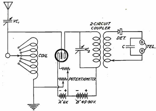
SINGLE-STAGE RADIO-FREQUENCY AMPLIFIER WITH CRYSTAL DETECTOR
