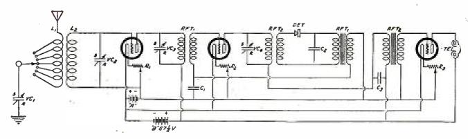
TWO STAGES OF TUNED-RADIO-FREQUENCY AMPLIFICATION, CRYSTAL DETECTOR AND TWO STAGES OF AUDIO-FREQUENCY AMPLIFICATION
