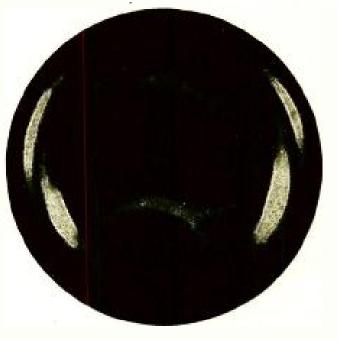
AN IMPERFECT RECEIVER The unsymmetrical arrangement of the sand shows that the receiver is not working correctly. Probably the poles of the magnet are improperly adjusted so that one is farther from the diaphragm than is the other.
