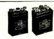
For low-voltage tubes Specially designed for WD-11 and UV-199 vacuum tubes, but can be used with any low-voltage tube. The two-volt Exide A Battery consists of a single cell. It will heat the filament of a WD-11 or other quarter-ampere tube for approximately 96 hours. The 4-volt A battery, having two cells, will light the filament of a UV-199 tube for 200 hours.
