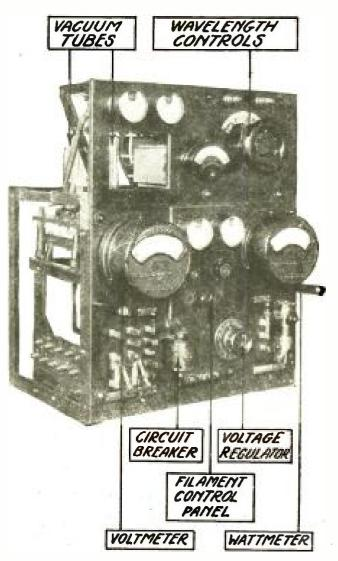
THE NAVY'S NEW TRANSMITTER This is the converted equipment which used to employ a spark but which now employs vacuum tubes that send out radio waves of exceptional purity.
