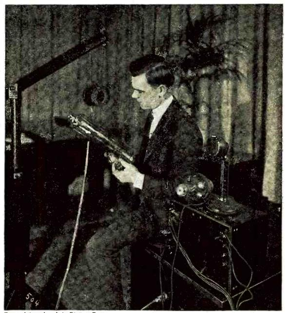
From a photograph made for POPULAR RADIO THE NEW VACUUM TUBE USED FOR BROADCASTING THE CONCERTS This triode was developed by the Westinghouse company for the express use of its broadcasting station. The old type of tube is shown at the elbow of the operator who is known to radio fans as announcer OBN of WJZ station.
