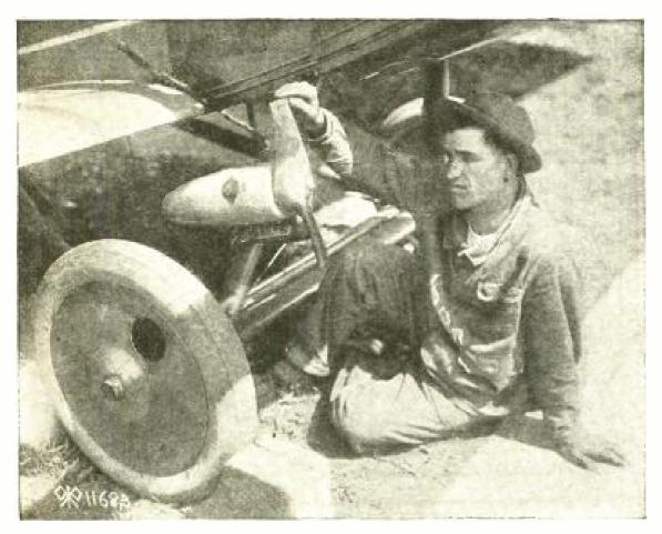
THE GENERATOR THAT SUPPLIES THE ELECTRICAL IMPULSE It is operated by a propeller-like fan beneath the fusilage; incidentally this device furnishes heat to the uniform of the aviator who flies in high altitudes.
