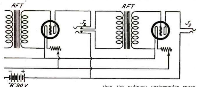
battery voltage should be used with it if it will work as an amplifier?
