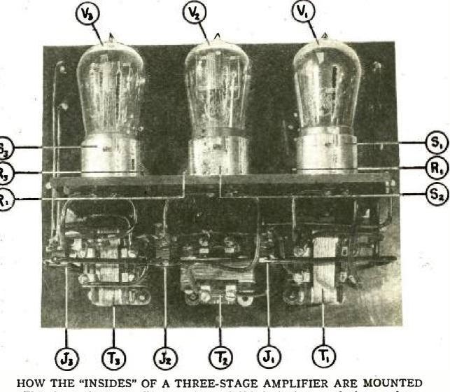
The tubes used are generally mounted on a shelf in back of the panel; they are shown here as  $V_1$ ,  $V_2$ ,  $V_3$ ; they are the tubes for the first, second and third stages, respectively. The sockets are designated as  $S_1$ ,  $S_2$  and  $S_3$ . Only a small portion of the three rheostats can be seen,  $R_1$ .  $R_2$  and  $R_3$ . The three amplifying transformers,  $T_1$ ,  $T_2$  and  $T_3$ , and the jacks  $J_1$ ,  $J_2$ ,  $J_3$ , are fastened to the panel underneath the shelf.
