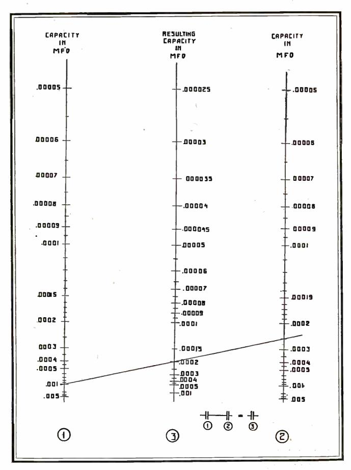
A CHART FOR CALCULATING THE CAPACITY OF CONDENSERS IN SERIES FIGURE 3. The capacity of two condensers connected in parallel may be easily found by adding the capacities of each of the condensers together, which will give the capacity of the whole. But to determine the capacity of condensers in series is a more complicated matter. This chart indicates the answer to this problem; by laying a ruler across, as indicated by the diagonal line, calculations may be made.
