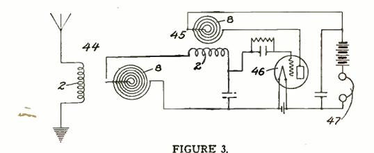
An interesting use may be made of two of these couplers, one as a tuner and the other as a feedback, as shown in this diagram of a regenerative circuit.
