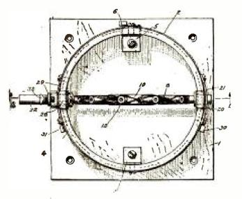
FIGURE 2 In this plan view the rotor is shown in the position of minimum coupling.
