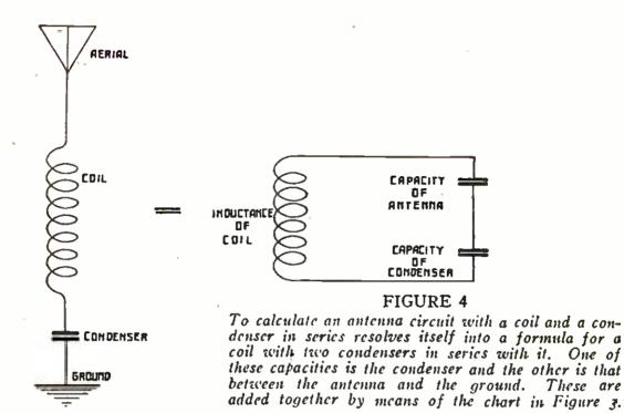
Find the correct value of inductance to use in a circuit shown in Figure 3 in which a condenser is placed in series with the antenna circuit, the antenna having a capacity of .00025 mfd. and the condenser a capacity of .001 mfd. to tune to 400 meters.
