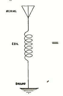
In order to illustrate the method of using this chart, let us take the following problem: In Figure 1 we have a coil connected in an antenna circuit. This circuit is equivalent to a coil with a condenser connected across it—the condenser in this case being the capacity between the antenna and ground.
