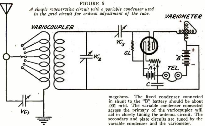
QUESTION: Kindly give me a good circuit that employs three .0005 mfd. variable condensers and a variometer, to be used with an audion detector.
