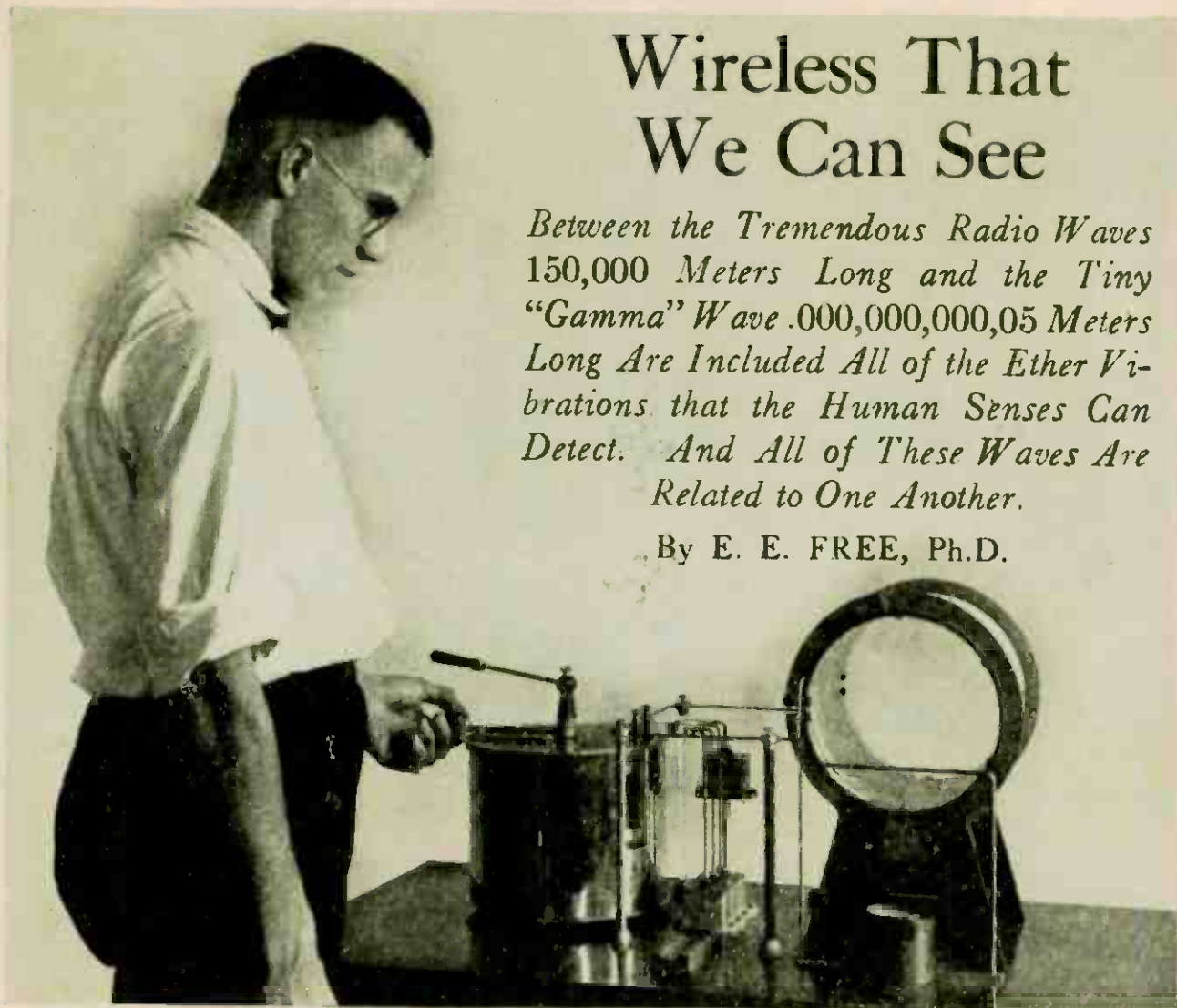
The wavemeter developed by the Bureau of Standards for measuring wavelengths.
