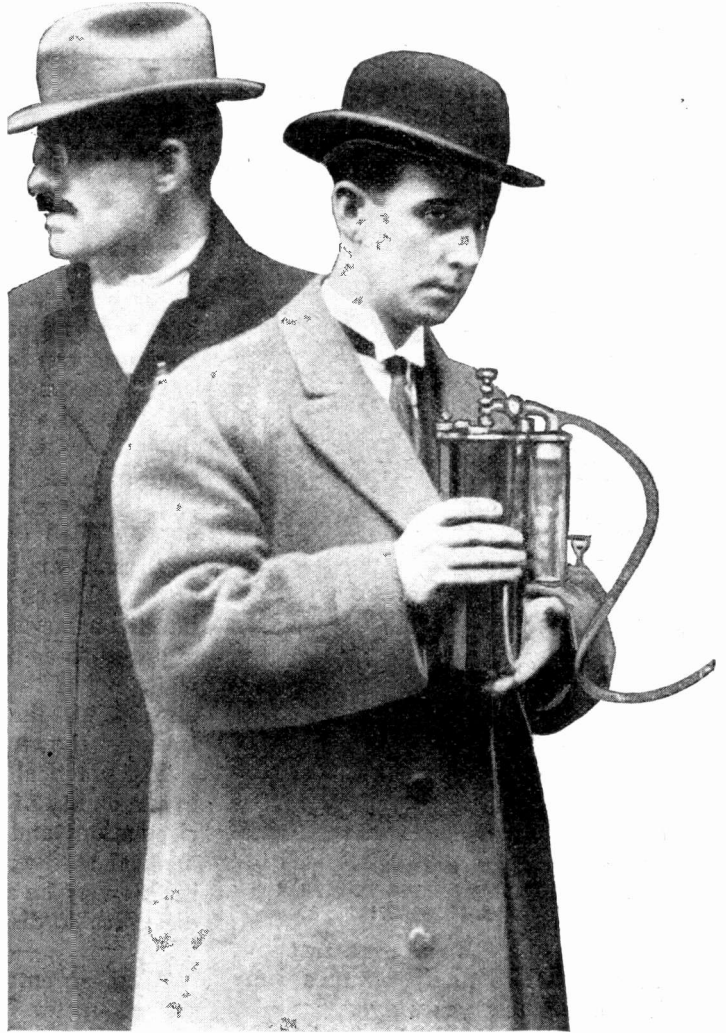
THE AUTOGENOR IS A VALUABLE AID TO FIREMEN WHO OFTEN MUST WORK WHERE THERE ARE POISONOUS GASES
