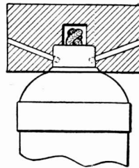
PLUG ARRANGEMENT FOR FASTENING SOCKET TO ARM
