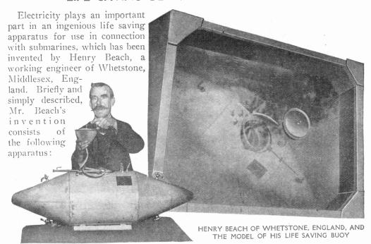
A well six feet across and 3½ feet deep is cut into the deck of the submarine near the conning tower and inside this is a watertight buoy, to which is attached a length of armored hose, including three strands of cable. The other end of this hose passes through the bottom of the well into the interior of the submarine and establishes communication with the buoy.
