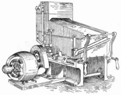
MACHINE FOR CRUSHING OATS
