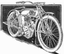
Mechanically oiled by THOR Perfection Force Feed Mechanical Oiler.
