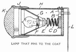
(G) is the reflector taken from the same light, while (K) is the lens and (F) a  $2\frac{1}{2}$  volt tungsten lamp, mounted exactly as in the flashlight.
