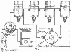
CONNECTIONS OF COMBINATION SPARK PLUG AND COIL
