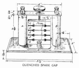
The lowest aluminum rod (G) is placed on this lower brass plate, a strip of mica 5% inch wide and long enough to reach from the center of one of the holes to the center of the other hole when the rods are arranged is placed on the top of the aluminum rod. The next rod (F) is placed on top of this, and so on with the remaining rods. In this manner the gap is built up and clamped by the thumbscrew.
