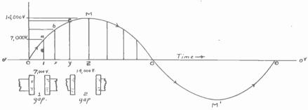
FIG. 7. DIAGRAM SHOWING THE RELATIONS BETWEEN CHARGING VOLTAGE, LENGTH OF SPARK GAP AND FREQUENCY
