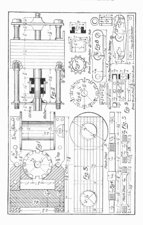
To insulate the armature cover the shaft next to the armature with 1/32 inch sheet fiber 3/4 inch wide. Make two 1/16 inch fiber washers 21/4 inches in diameter, slip them on the ends of the shaft and glue them to the ends of the armature. After the glue has set cut out the slots. Make twelve channel pieces out of 1/32 inch sheet fiber and glue them into the slots and to the fiber washers; when set trim off with a sharp knife and be sure to have all the iron covered.
