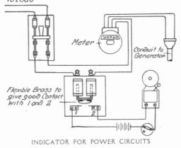
armature is drawn up into the coils by the current flowing through them. The moment the load goes off and there is no current flowing in the line the Ushaped piece drops upon the two brass contacts, (1) and (2), closing the battery circuit and ringing the bell.—MARSHALL S. LOKE.
