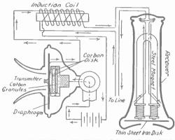
FIG. 4. ESSENTIAL FEATURES OF A TELEPHONE TRANSMITTER AND RECEIVER
