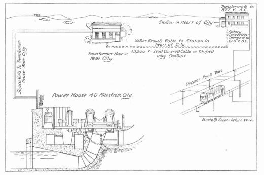
FIG. 1. GENERAL SCHEME OF A POWER TRANSMISSION AND RAILWAY SYSTEM
