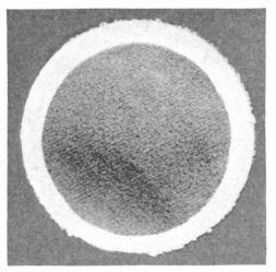
A PIECE OF FILTER PAPER THROUGH WHICH THE VOLUME OF AIR BREATHED BY A MAN IN 24 HOURS HAS BEEN DRAWN
