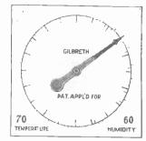
SPECIAL CHRONOMETER WITH LONG HAND MOUNTED BE-SIDE THE WORKMAN AND APPEARING IN EACH PIC-TURE OF THE FILM
