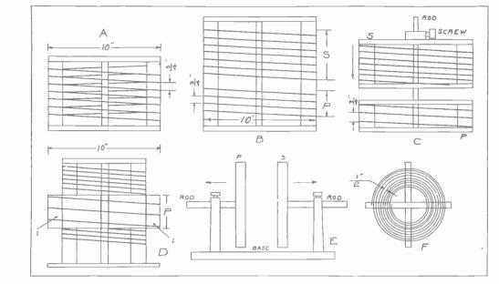
FIG. 6. TYPES OF OSCILLATION TRANSFORMERS
