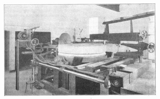
GRINDING THE MIRROR OF A 100 INCH TELESCOPE
