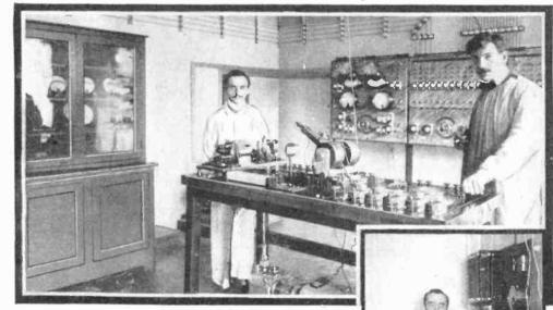
AT THE TOP OF THE PAGE IS SHOWN A RECEIVING CYLINDER BEARING A PICTURE SENT BY WIRE FROM BORDEAUX TO PARIS IN FOUR MINUTES; IN THE CENTER, COMPLETE SENDING APPARATUS IN DR. BELIN'S LABORATORY
