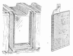
FIG. 6. CROSS SECTION AND ONE PLATE OF A STORAGE BATTERY
