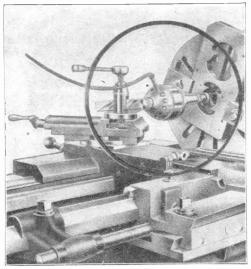
PORTABLE GRINDER FOR MACHINE TOOLS
