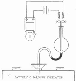
mercury is in connection with the space above the battery, which is enclosed. When the charging is complete and gas in excessive quantities begins to be given off, the pressure pushes the mercury in the tube until it forms a connection between two wires which form part of the circuit of an electric bell. A sort of safety valve is also provided for the escape of any accidental sudden pressure, caused for instance by the pressure of the stopper or by the sudden expansion of heated gas.
