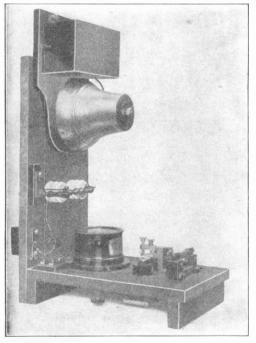
FIG. 1. NEW TELEFUNKEN APPARATUS FOR DETECTING THUNDERSTORMS
