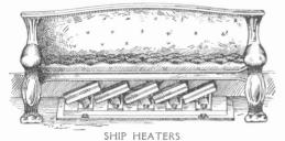
The pedestal heaters can be used singly in a stateroom or in groups of two or three for saloon heating. Another way is to mount a series of heaters under seats as shown and in this case they can be located in a low space.
