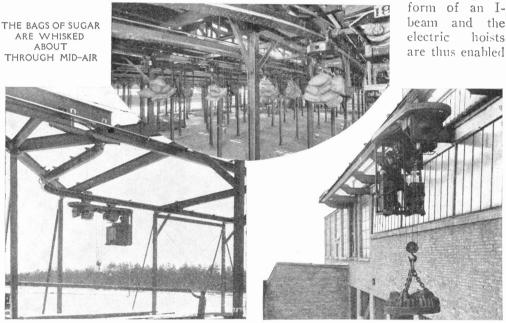
FLEXIBLE METHOD OF SWITCHING IN MONORAIL SYSTEM
