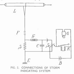
known, the distance of the thunderstorm can be gauged by measuring up the paper tape and counting the number of points recorded thereon.
