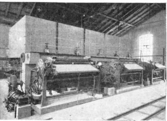
SEPARATOR WITH DISTRIBUTING TANKS BEHIND
