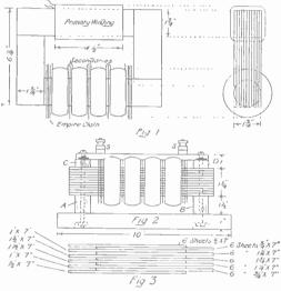
DETAILS OF CLOSED CORE TRANSFORMER
