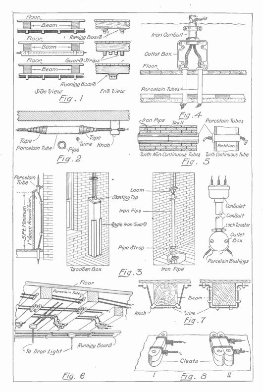
ever, iron pipe is considered preferable to wooden boxing and its use is strongly urged. It is especially suitable for the protection of wires near belts, pulleys, etc. Fig. 4 shows an outlet arrangement with a square conduit outlet box at the floor.
