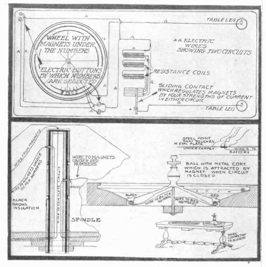
LAYOUT AND CONNECTIONS OF THE CROOKED ROULETTE WHEEL
