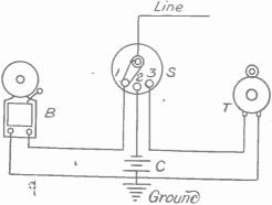
CONNECTIONS FOR SIMPLE TELEPHONE SYSTEM
