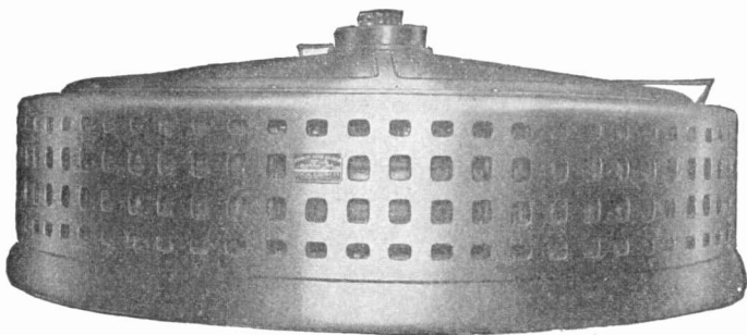
ONE OF THE KEOKUK GENERATORS WHICH MEASURES 30 FEET IN DIAMETER AND WEIGHS OVER 600,000 POUNDS
