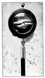
DETECTOR FOR LIVE WIRES
