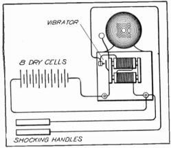
FIG. 2. SUBSTITUTE FOR SHOCKING COIL
