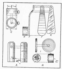
FIG. 2-DETAILS OF GALENA DETECTOR
