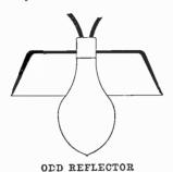
of men in a deep ditch at night. A hole was punched through the bottom of an ordinary tin basin, the wires attached and the current turned on. The device was rigged up in a moment and was as good as anything could be for the work required.
