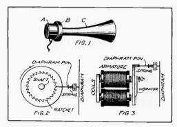
PARTS OF AN ELECTRIC AUTO HORN
