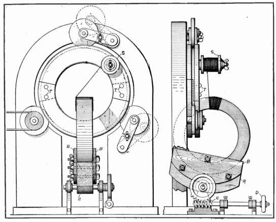
MACHINE FOR WINDING RING ARMATURES
