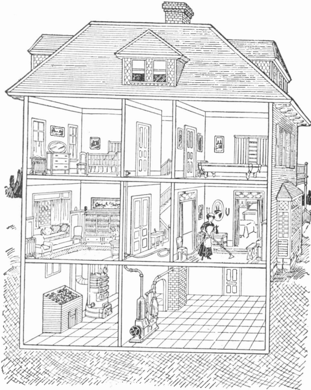
HOUSE PIPED FOR VACUUM CLEANING
