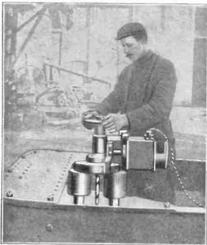
FIG. 2. ELECTRO-MAGNETIC DRILL FOR BENCH WORK
