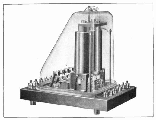
FIG. 7. COMMON FORM OF "RELAY" USED IN ELECTRIC BLOCK SIGNALING
