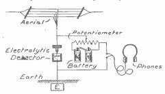
FIG. 114. CONNECTIONS FOR ELECTRO-LYTIC DETECTOR
