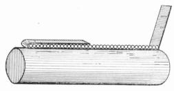
METHOD OF WINDING MAGNET COIL
