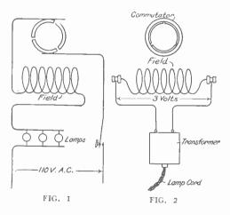
most suitable for the purpose is the small three-pole armature type. Fig. 1 shows the connections of such a series wound motor for operating in series with three sixteen candle-power lamps in multiple.
