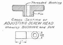
FIG. 110. DETAILS OF SCREW HEAD AND BUSHING
