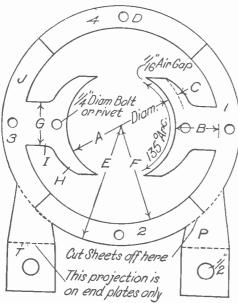
FIG. 8. FRAME OF TWO-POLE DYNAMO OR MOTOR
