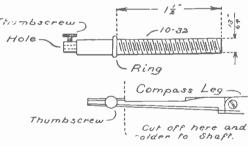
FIG. 122. SHAFT FOR HOLDING WIRE
