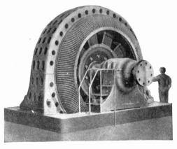
GENERATOR OF 8,700 HORSEPOWER
