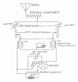
FIG. 6. RECEIVER CONNECTIONS
