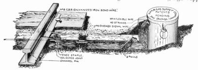
FIG. II. CONNECTIONS BETWEEN TRACK CIRCUIT AND BATTERY CHUTE
