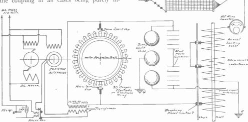
FIG. 5. DIAGRAM OF SECONDARY CONNECTIONS
