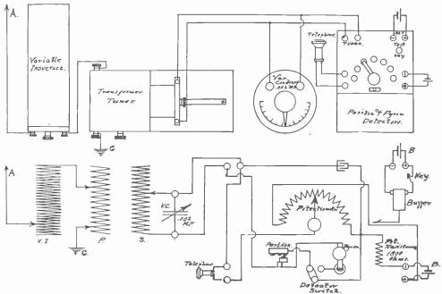
FIG. 7. DIAGRAM OF UNITED STATES NAVY STANDARD I. P. 76 RECEIVING SET
