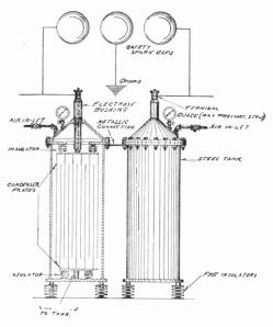
FIG. 4. SIDE VIEW AND CROSS SECTION OF CONDENSER
