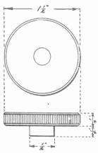
FIG. 118. ADJUSTING SCREW HEAD
