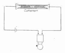
metal filings between the ends of brass rods just fitting the tube. The filings and rods are connected in series with a battery and bell. Wireless waves will cause the filings to "cohere" thus reducing the resistance of the circuit and operating the bell, the hammer of which taps the tube and places the filings in a disturbed state again. (See cut.)
