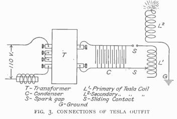
inches long made of dry birch boards glued together in a circle and then turned off in a lathe. The turns of wire are carefully spaced apart 1-16 inch when winding, leaving a margin of  $\frac{1}{2}$  inch on the ends. The primary is wound on a wooden drum eight inches in diameter and  $4\frac{1}{2}$  inches long, the turns being carefully spaced apart and fastened. The secondary coil is set on top of the primary coil and the base fastened to the bottom drum.
