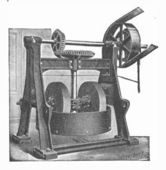
CRUSHING MACHINE FOR GRINDING UP THE CRYSTALS
