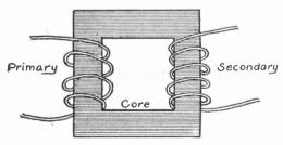
FIG. 92. SIMPLE TRANSFORMER WITH RECTANGULAR CORE
