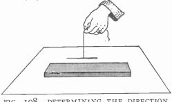
FIG. 108. DETERMINING THE DIRECTION OF MAGNETIC FIELD
