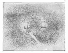
FIG. 111. PIECE OF IRON IN MAGNETIC FIELD
