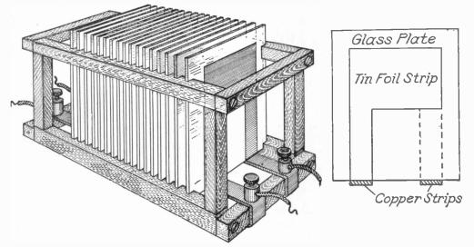
FIG. 2-CONDENSER FOR HIGH FREQUENCY APPARATUS
