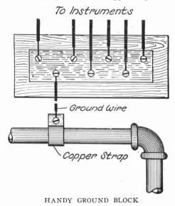
doing this. Take a piece of sheet brass about 1 by 4 inches and bore several 3-16-inch holes in it for round-headed brass screws. Fasten this plate to a hard wood block on the wall and connect to a water pipe if possible. Any instrument that you wish to ground may then be easily connected by wire under one of the screws of the ground plate. This device should be used only where very small currents are involved and if possible a slate block provided in place of the wood.
