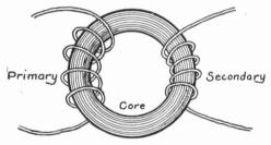
FIG. 91. SIMPLE TRANSFORMER WITH RING CORE
