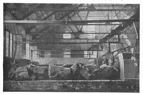
CARBORUNDUM FURNACE AFTER BURNING, SHOWING CRYSTAL MASSES
