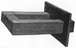
FIG. 99. CORE WITH HEAD SLIPPED ON
