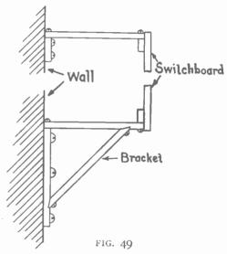
Construct two brackets, from some oak pieces three inches wide, as shown in Fig. 49 that are to serve as supports for the switchboard. Two other pieces 18 inches long, three inches wide and  $\frac{7}{8}$  inch thick may be used at the top to steady the board. The figure shows a side view of a board supported as just described.
