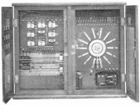
TESTING APPARATUS FOR AUTOMATIC JOURNAL ALARM
