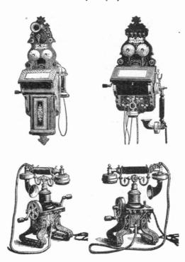
scribers' telephone sets used in Sweden. The handsome wood carving and inlaid decorations are foreign to American instruments, while the connecting of receiver and transmitter is unusual except on testing out-
