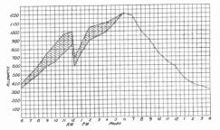
FIGS. 164 AND 165. LOAD CURVES OF LIGHTING STATIONS, SHADED PORTIONS SHOWING LOAD DUE TO ELECTRIC IRONS
