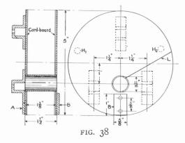
inch wall. Cut from some 1-16-inch sheet brass two circular pieces five inches in diameter. Make an opening in each of these pieces one inch from their center and of such a size that they will slip on the ends of the brass tube. Cut from some \(\frac{1}{8}\)-inch brass two pieces one inch long and \(\frac{8}{2}\)-inch wide.
