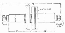
FIG. 13. DETAILS OF BUSHING
