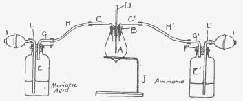
FIG. I. APPARATUS FOR MAKING SAL AMMONIAC
