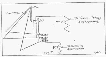
FIG. I. ARRANGEMENT OF THE DIRECTIVE AERIAL
