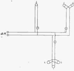
FIG. 13. BRANCH LIGHTING CIRCUIT AND SNAP SWITCHES
