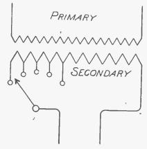
FIG. 19. HOW TAPS ARE TAKEN FROM THE SECONDARY
