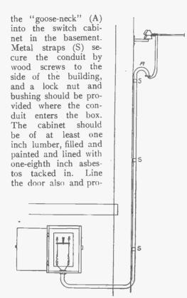
FIG. I. SERVICE WIRES AND SWITCH
