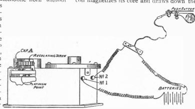
HOW THE AUTOMOBILE HORN IS CONNECTED
