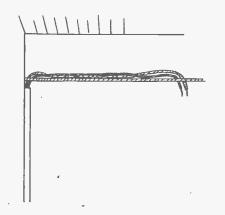
FIG. 9. FISH AND MOULDING WORK COM-BINED .
