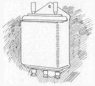
TRANSFORMER TO OPERATE ELECTRIC BELLS
