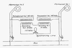
SCHEME OF PARALLELING ALTERNATORS
