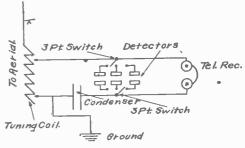
CONNECTIONS FOR TESTING CRYSTALS
