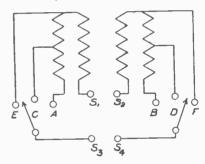
FIG. 23. ARRANGEMENT OF TAPS FROM THE SECONDARY
