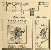
Circuit and Arrangement of Lamps
