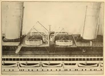
Collapsible Boats Nested Between the Funnels of the S. S. Imperator, Arranged to Economize Space
