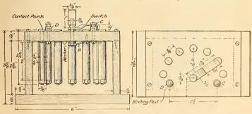
Interior and Top View of Rotary Potentiometer
