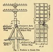
has a much greater tendency to steady the pole than would a number of guys. Another thing in connection with the use of this style of construction is that it is sometimes possible to find a dry spot here and there through a bit of
