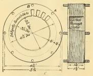
Fig. 1. Stator of Mctor
