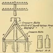
Fig. 2. Stubs to Support Pole
