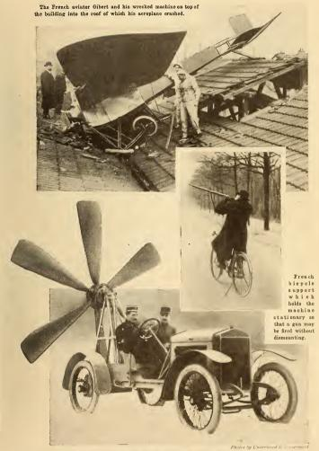
The latest addition to the transportation facilities of the French army is the flying auto. Note monster propeller attached to rear which helps auto to attain speed of 50 miles an hour over desert sands.
