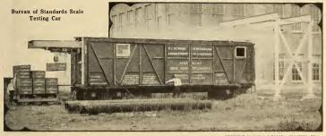
different cities of the union. The car, as is shown in the illustration, is equipped with a number of standard weights, and apparatus for putting them on the track scales to be tested. A crane bridge equipped with a trolley and a hoist can be projected out of one end of the car and any given number of standard weights can be placed on the small truck and run out on the scale platform.
