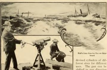
shifted to any direction or angle of clevation necessary, and two minutes after the gun is set on the rail, the shot is carrying the line out and over the distressed vessel.
