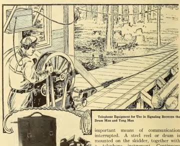
ly between the drum man who controls the big cable winding drum and the tong man in the woods who attends to the log tongs on the skidway is imperative. Here the telephone, of an unusual type, steps in as a refinement over the old method of signaling by lung power or gesticulations, by whistles, strings and cords; in fact, every method that had before been conceived.
