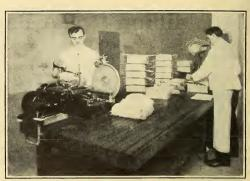
All Day Long One Man Slices Ham for Sandwiches, with an Electric Slicing
