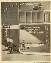
Compressed Air in The Hold of the Ship Prevents the Water from Entering
