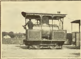
Curious Hot Water Engine Used on Some of the Street Railway Lines in Weltevreden
