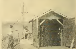
Vertical, Fifteen Horsepower Motor Driving a Six Inch Pump to Irrigate 40 Acres of Alfalfa
