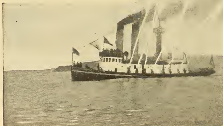
One of San Francisco's New Fire Tugs Delivering a Broadside of Eight High Power Jets
