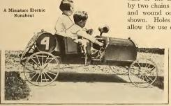
Master Tom Hoyt, son of the well known consulting engineer of Cleveland. The little car is complete to the last detail, is driven by a small electric motor with clutch and two brakes and has a dummy shift lever. The driver of the car will never be molested for exceeding the speed limit of most cities, as the greatest speed to be obtained is but six miles per hour. It has been considered the most practical and complete little car ever constructed.
