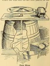
barrel, they must be stirred for about ten minutes. Then the stirring outfit can be lowered into the barrel, the rim of the wheel resting on the pulley of the motor.—WILSON S. SUIFIN.
