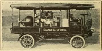
A Compact Equipment for Thawing Frozen Waterpipes by Electricity
