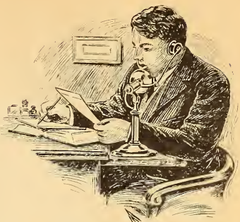
Telephone Receiver that Need not be Held in the Hand
