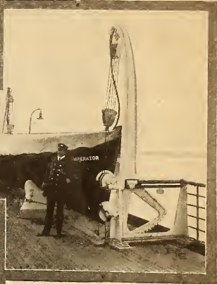
The winches shown at the left, and operated by electric motors, are used as baggage and mail hoists, also for lifeboats.
