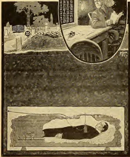
SUGGESTED METHOD OF ARRANGING A GRAVE ALARM
