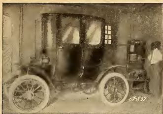
CURRENT CONVERTER IN PRIVATE GARAGE
