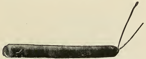
FIG. 18. COMPLETED CORE AND PRIMARY
