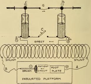
FIG. 12. DIAGRAM OF HIGH FREQUENCY APPARATUS.
