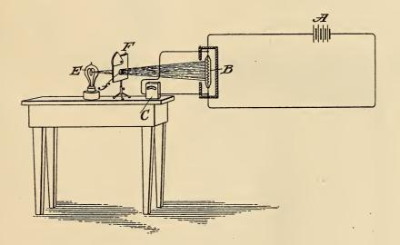
tice to compare the intensity of light which it gives with that given by a standard lamp of known candlepower. Such tests, however, have the disadvantage of the fallibility of the human sight. No two persons see exactly alike and therefore photometer tests or comparisons made by different persons may not agree.
