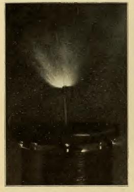
FIG. 2. DISCHARGE OF A TESLA COIL.
