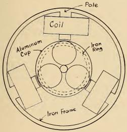
frame with three iron poles projecting inwardly very close to the disk. The poles should be 120 mechanical degrees apart.
