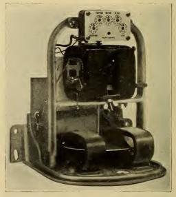
FIG. 30. RECORDING WATTMETER.
