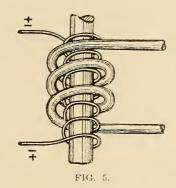
electrodes and contacts are avoided in apparatus of the transformer type. Electrical energy is most economically conveyed over long distance in the form of alternating currents of high voltage and small volume, and these currents are converted into alternating currents of low voltage and great volume by means of "step down" transformers, inserted between the line wire and the groups of lamps or motors which they supply. Such
