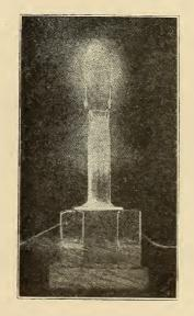
Compared with ordinary lamp filaments, the Helion filament is considerably thicker and stiffer, but in spite of this its resistance is so great that only a short filament is required.
