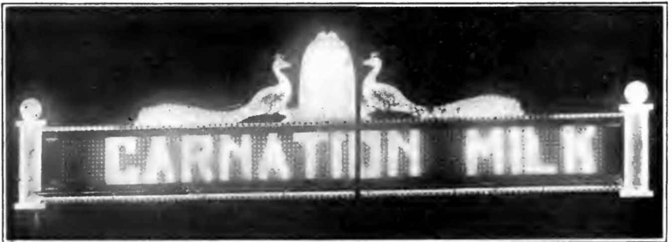
Perforated Paper Rolls Serve to Change the Lettering on This Attractive Electric Sign. From One to Sixty Words per Minute can be Flashed on the Bulletin Board.
