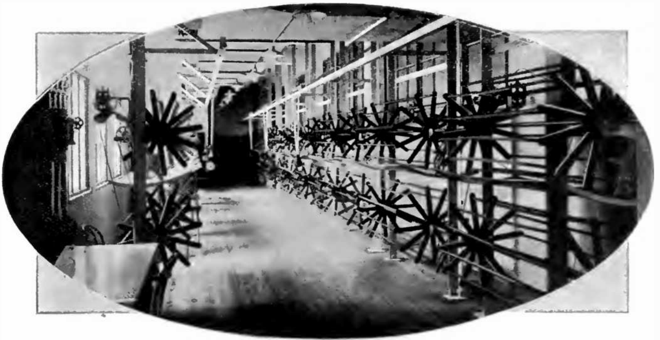
On These Wooden Frameworks the Wet Film is Wound and Then Revolved Until it is Thoroughly Dried. The Room is Heated at a Uniform Temperature to Expedite the Work.
