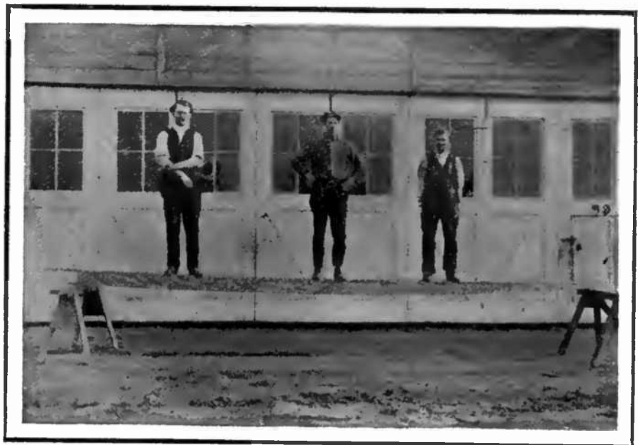
Capable of Withstanding the Weight of Three Men, this Aeroplane Girder is Extremely Light in Weight.
