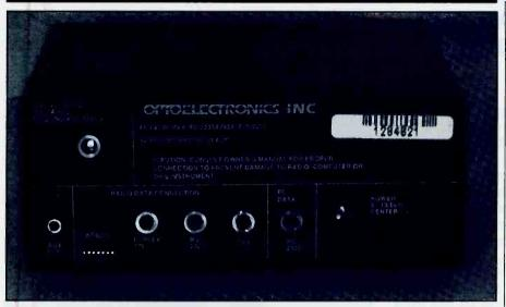
A myriad of connections is available on the rear panel, but unless you're using the unit under computer control, you'll only need power and audio at the upper left. Note the AR-8000 ribbon connector at the bottom left.
