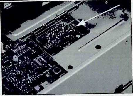
Some scanners, like the popular BC-9000 from Uniden, need an optional CTCSS board installed before they can take advantage of tone squelch. Note that the 9000 only does CTCSS even with the board — DCS is not available.
