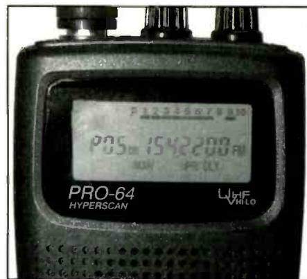
The unique priority system on the PRO-64 and 2041 allocates a special priority bank of 10 channels. This allows for priority channels in use to be consistent, no matter what banks you're scanning, but also takes some time to cycle through the entire bank.
