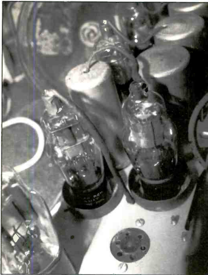
The 42 audio PA has been removed to show the new shielded grid lead assembly. Note how those tubes shine after being cleaned!
