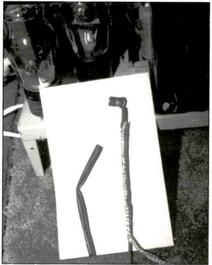
The shielded braid is snaked over the grid wire, and will be grounded below chassis. The heatshrink tubing has yet to be applied to hide the shielding.
