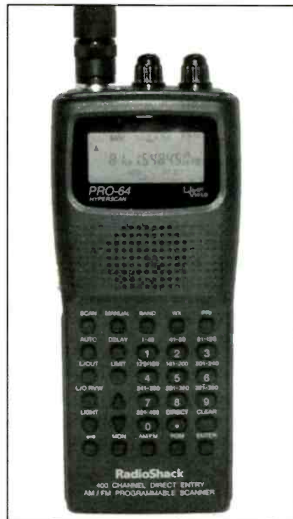
The handheld PRO-64 is the first RadioShack scanner offered with a computer interface, although it was a well-kept secret. The interface only supports downloading frequencies, but that function alone is a real timesaver!
