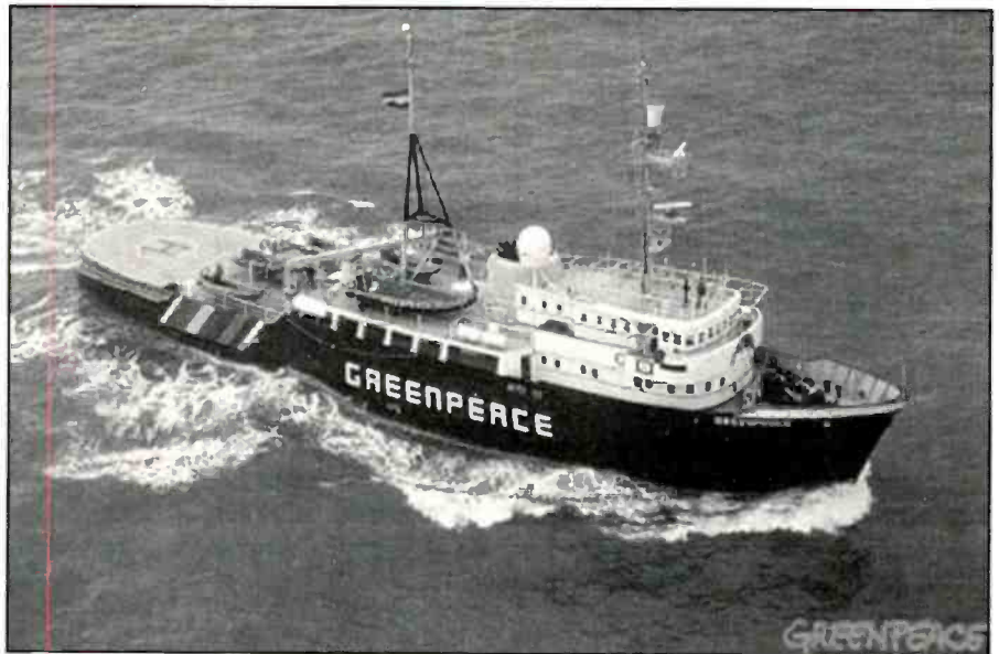
Another member of the Greenpeace fleet is the M/V Greenpeace, seen here after installation of an aft helo pad in 1986. (Photos courtesy Greenpeace)
