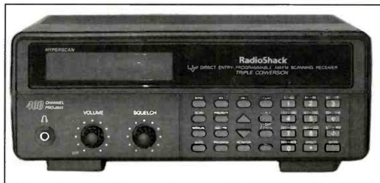
The PRO-2041 base unit is functionally identical to the handheld. Both receivers are triple conversion design and are relatively free of unwanted signals. The 2041 front panel is almost identical in size to the older 2006, although the cabinet is not quite as deep.
