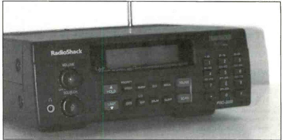
The 2050 is housed in a small cabinet, making a nice, compact unit for either home or mobile operation (the mobile mounting bracket is not supplied).
