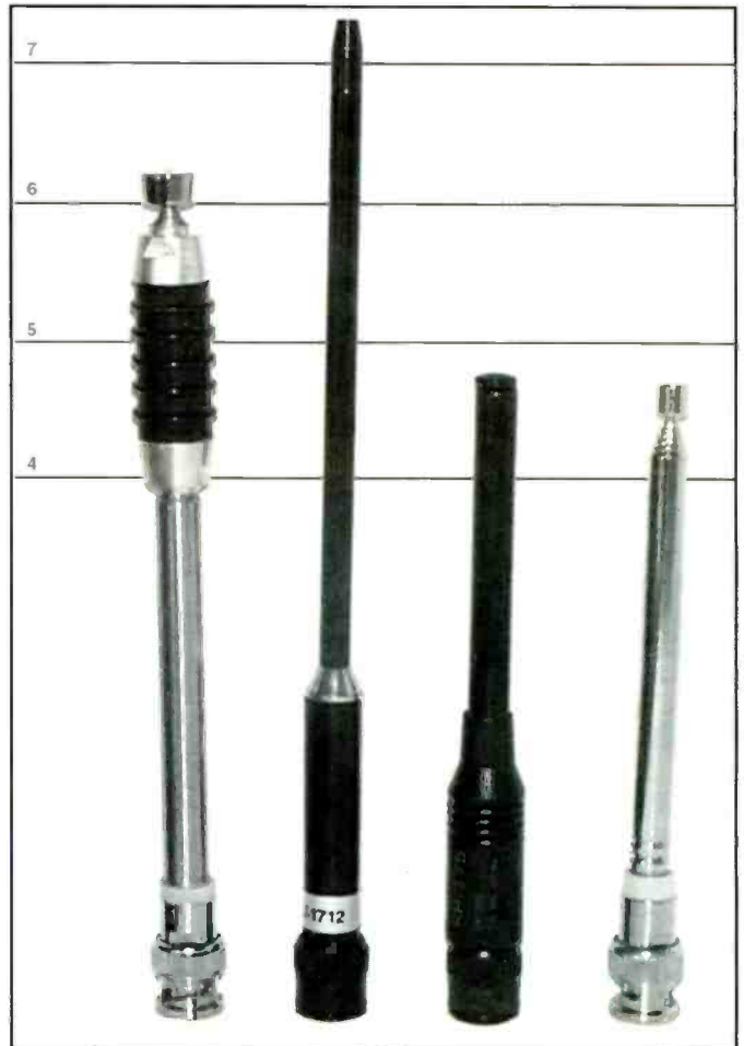
When reduced performance is acceptable, or shorter range is desirable, these short antennas are easy to hide and carry. Shown are the Maldol Active Hunter AH-209S, a UHF-only antenna (sorry, I can't identify the manufacturer) which provides great performance on UHF (and reduced sensitivity on VHF and 800), and the Comet DB-32, the ultimate small antenna. Check your favorite radio dealer for these, or similar antennas for your handheld.
