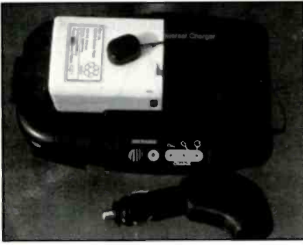
The battery pack sits flat on the charger to pick up the gold pin contact points. A strong magnet inside the charger holds the pack in place, while a sensor to detect heat sits on top of the battery.
