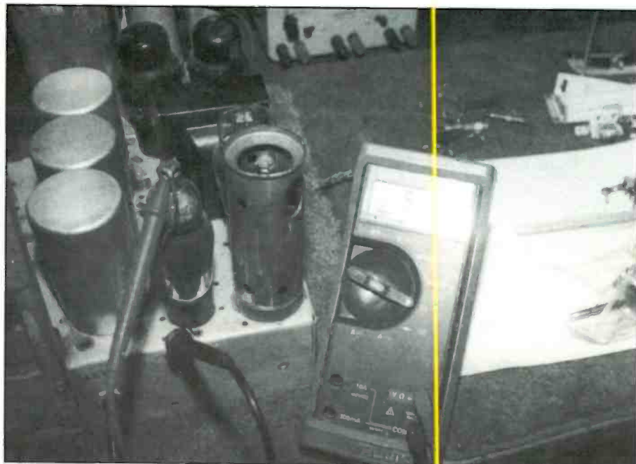
Here's Peter's Fluke 77 being used to do some basic troubleshooting in this Philco chassis.
