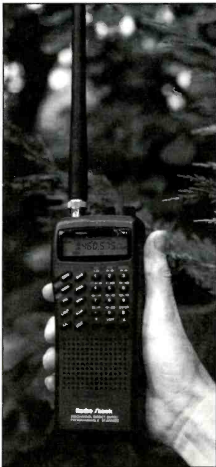
The small rubber duck antenna on scanners like this RadioShack unit will provide good reception: in some areas, if you're close to the action, you might even want to remove the antenna to be more inconspicuous.
