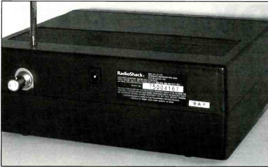
The rear panel of the 2050 is straight to the point. Note the 12-Vdc connector for use with the included wall transformer, or mobile power source.
