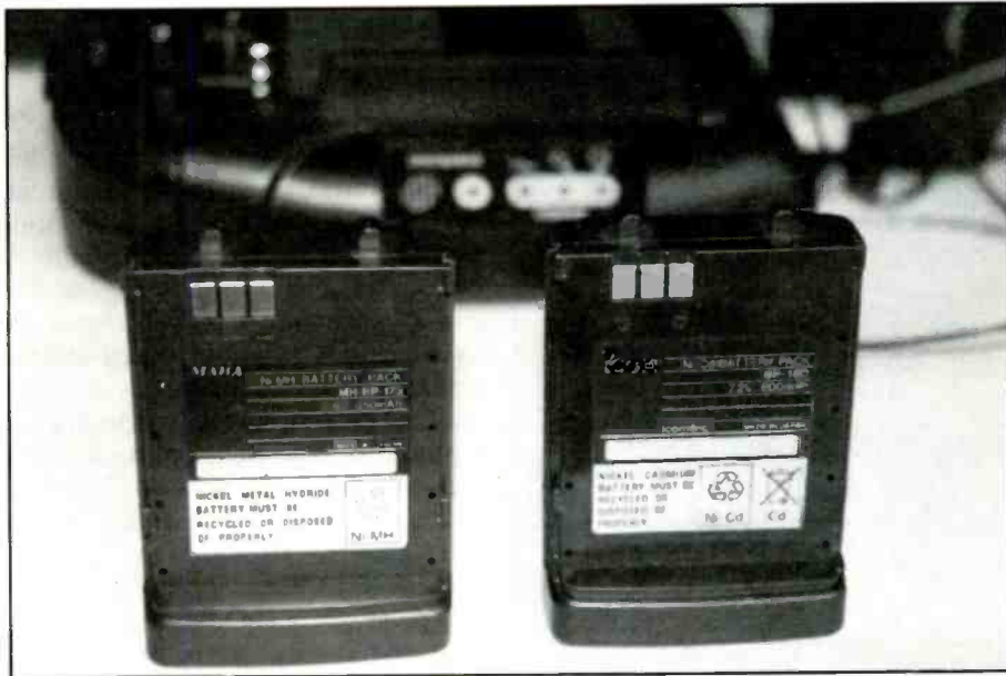
The NiMH battery on the left has almost twice the capacity as the NiCd on the right.
