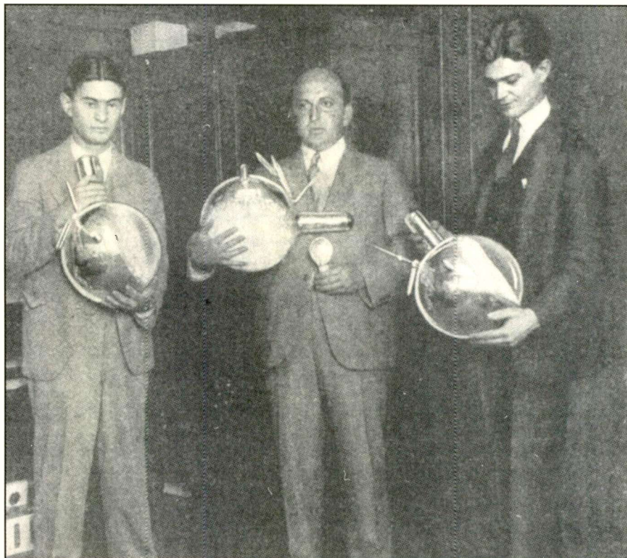
Three giant photoelectric cells used in 1928 by WRNY/W2XAL, the first television broadcast station, are proudly displayed. Pictured here, from left to right, are WRNY's Bob Hertzberg (W2DJJ); Pilot's President, Isidor J. Goldberg; and John Geloso, the engineer who designed the pioneering television equipment.
