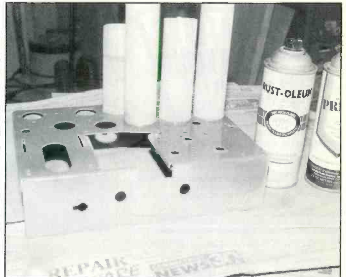
The chassis was finished with two coats of gray primer, followed by two coats of zinc-bearing paint.
