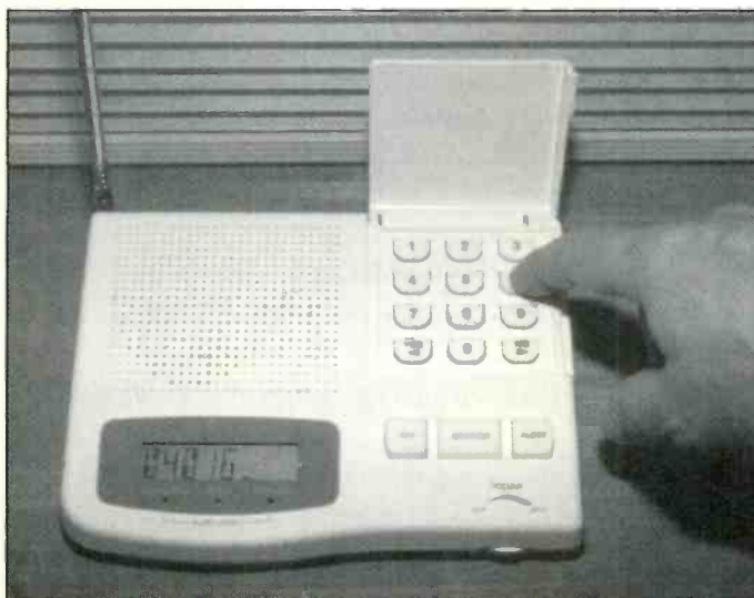
The RadioShack 7-Channel Weatheradio being programmed with FIPS code for SAME operation. (Photos by Keith Brewster)
