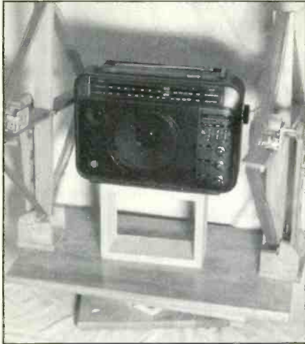
A GE Super Radio III with the assembled loop and turntable.
