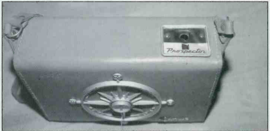
[TOP VIEW] Above the metal plate bearing the “Prospector” legend is a peephole for viewing the neon bulb for a visual indication of radiation. The push-button for charging the Geiger tube is also on this plate. The leather case and carrying strap show no signs of wear, and the stitching is in excellent shape. This set is about as close to a “10” as you will find.
