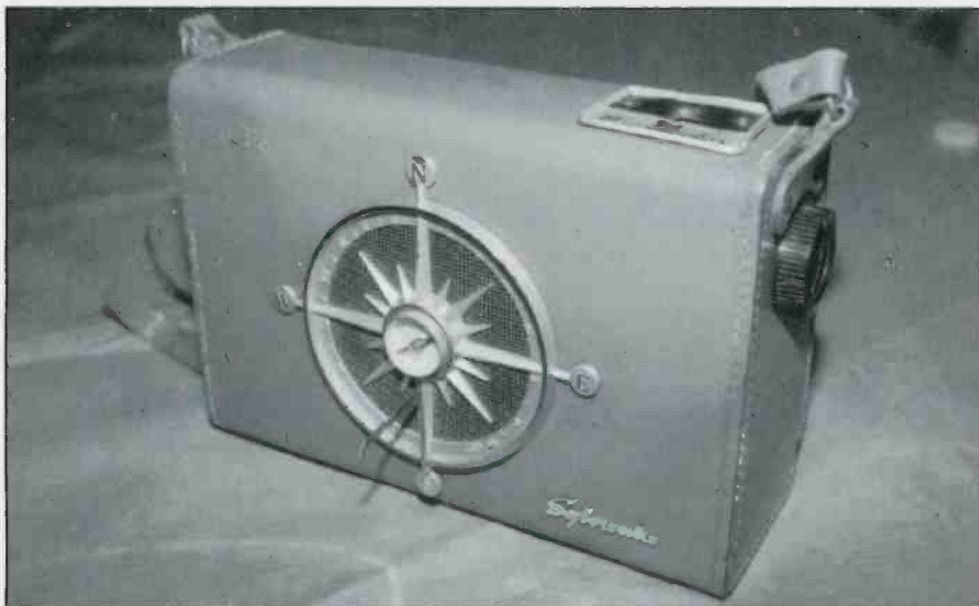
The Sylvania model U235 "Prospector." A rare radio relic from the Cold War era. Notice the compass at the center of the sundial rosette. The sundial forms a clever grille for the speaker. Sundial arm is extended, and the volume control is visible at the right side. The tuning knob is on the opposite side.
