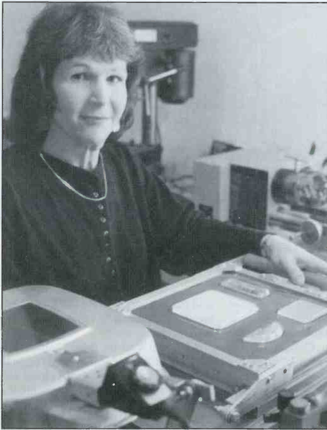
← Rita at work! Various shop tools in background are used to make the custom molds for the dial covers. In front of Rita is a vacuum heat table used to form the plastic over the molds.
