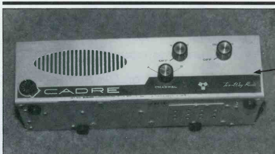
If your Cadre is a 510A it will have a tunable receive knob located here.
