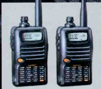
FT-10/40R Ultra Compact Handhelds VHF or UHF. Similar to FT-50RD including MIL-STD 810, and other exclusive features.
