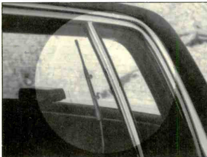
If a low profile is desired for any communications equipment, this inside-the-glass suction-cup cellular antenna can be hidden inside the surveillance vehicle. And with dark glass in therear windows, it would be hard to see it in actual use.
