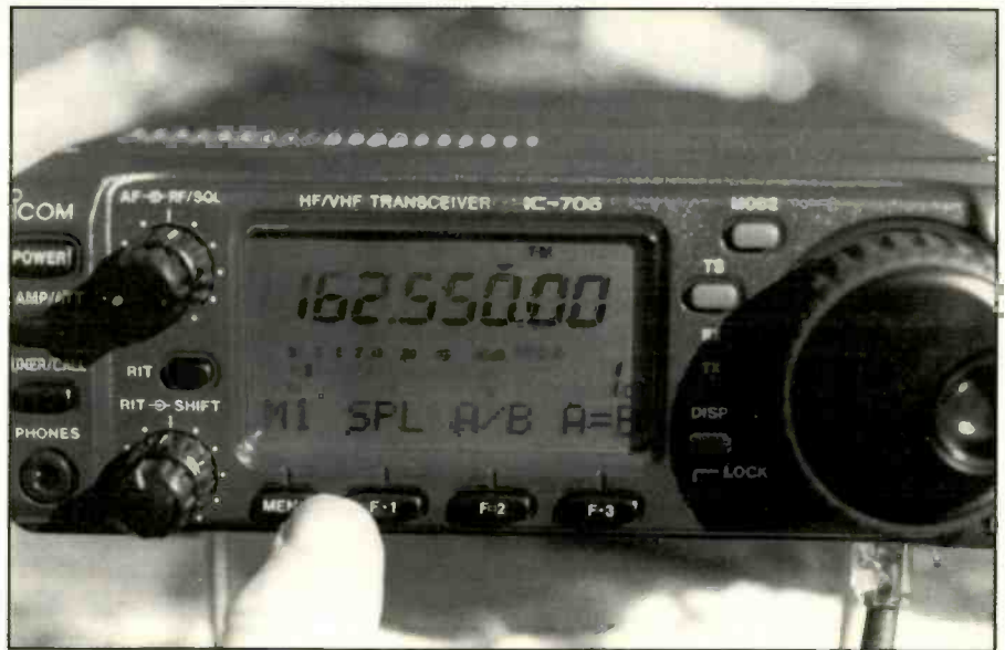
Tropospheric ducting can be identified by tuning in a distant weather station and hearing how strong it is.
