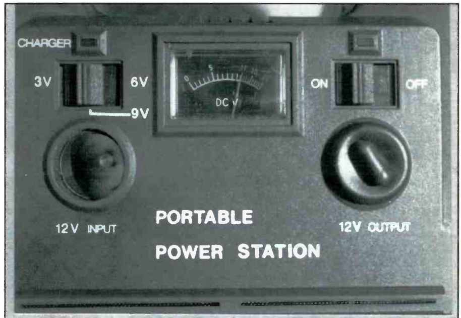
The portable Power Station has a hard-to-see meter with an illogical 0-20-volt scale.
