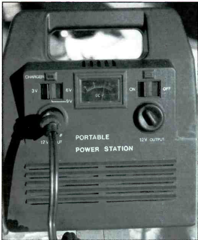
The left 12-volt input jack needs to be rewired to the 10-amp fused battery direct—not through the regulator.
