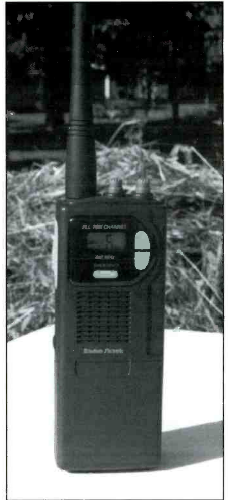
RadioShack's PRS-101 GMRS handheld radio operates on 10 UHF frequencies. (Photo by Chuck Gysi, N2DUP)
