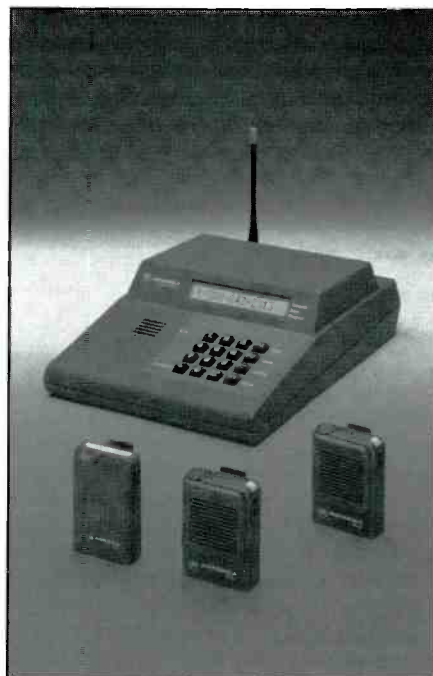
The Motorola CourtesyCALL was designed with a vibration-only alerting system. It advises waiting customers when their orders are ready. (Photo courtesy of Motorola)
