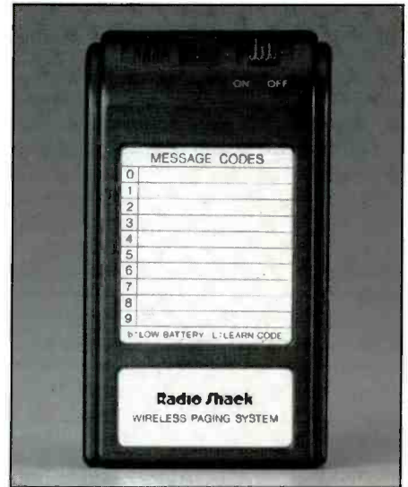
A close look at the beeper that comes with RadioShack's inexpensive on-site paging system. Users assign their own meanings to the 10 different message codes the system transmits.
