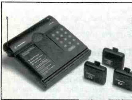
The Motorola CourtesyCALL was designed with a vibration-only alerting system. It advises waiting customers when their orders are ready. (Photo courtesy of Motorola)
