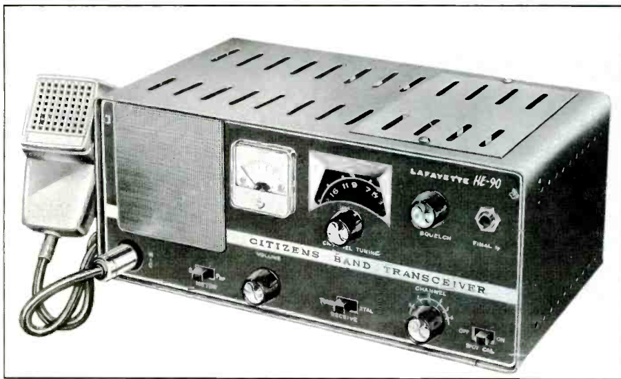
The Lafayette HE-90 was a late-1963 USL creation. It transmitted on six channels. The receiver had a Nuvistor front end.
