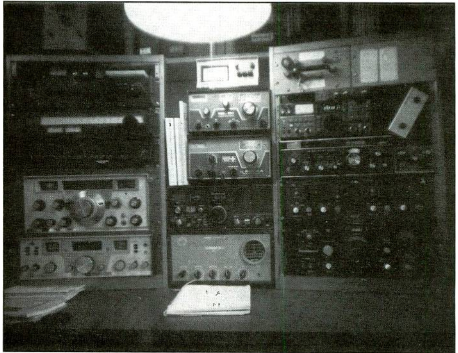
Here's the monitoring post of Brendan Boomer in New Jersey. This impressive line-up includes these receivers: a National HRO-500 and HRO-600, Drake SPR-4, SW-4 and R7, an Icom R-71 and a Collins 51S1 and associated panadaptors, distribution amplifiers, antenna rotator. Whew!
