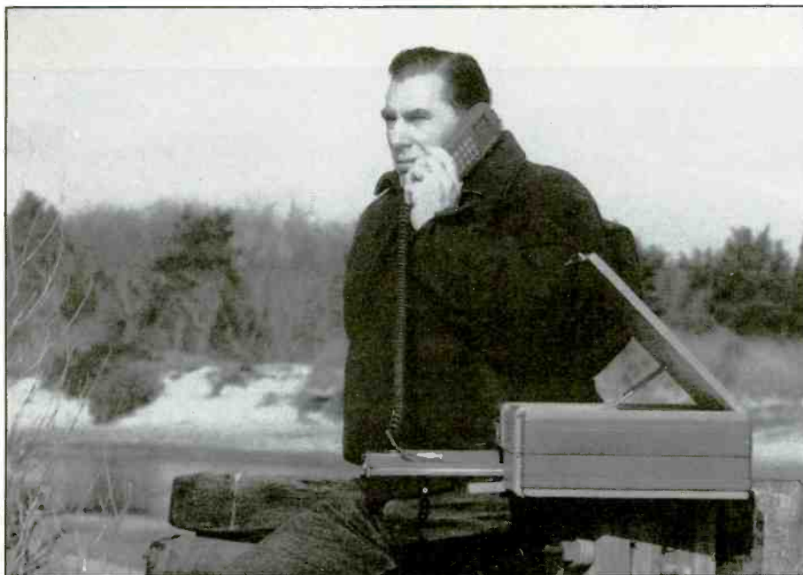
Maganavox MX-3030 portable satellite digital phone weighs 27 lbs., and is used with the MARISAT-M satellite. The mil spec unit can be used on land or sea for SAR missions. It's made by Magnavox/NAV-COM, P.O. Box 650, Deer Park, NY 11729.
