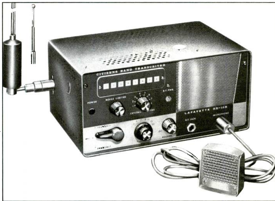
Lafayette's HE-15B was made in mid-1962 by USL. It had eight transmit channels. The IF frequency was changed to 455 kHz from the earlier version's 1750 kHz. Set sola for $59.50.
