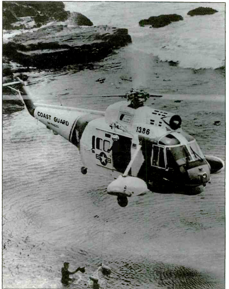
A Coast Guard Sikorsky HH-52A Sea Guard SAR helicopter on the job. (Coast Guard photo.)
