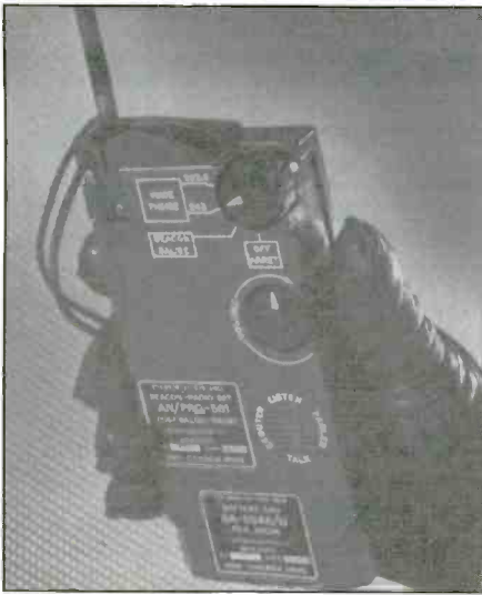
The ANPRQ-501, made in Canada by Garrett Manufacturing Ltd., Rexdale, Ont., sends out rescue beacon signals and voice on 243.0 and 282.8 MHz. It is intended to allow SAR units to locate downed military aircraft crew members.
