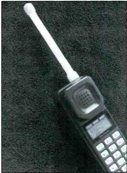
The Alter Systems Iso-Antenna is claimed to reduce radiation, while still producing a 3 db signal gain.
