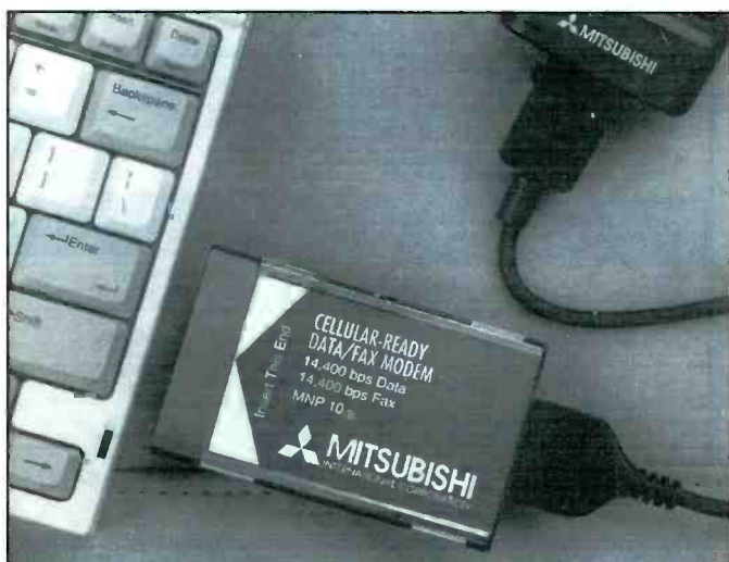
Mitsubishi introduced this portable data link that allows data or FAX to be transmitted over a handheld cellphone.
