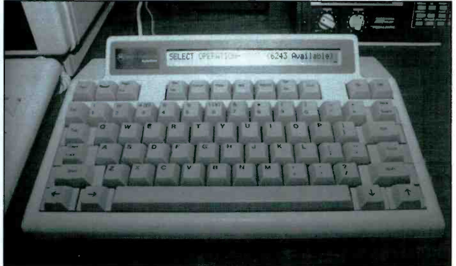
A look at the alphanumeric paging terminal used by Denver's Mountain News Net.
