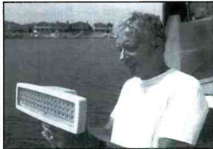
Author Gordon West adjusts his SART testing equipment to measure SART signal levels at 10 GHz.
