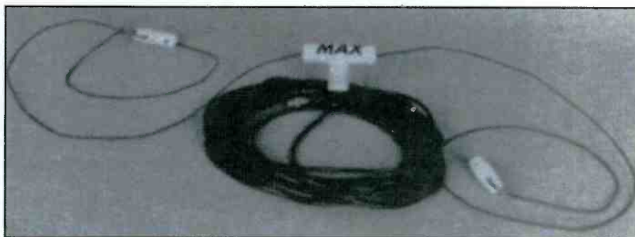
The Cellular Security Group's 49 MHz dipole as it appears before it's installed.
