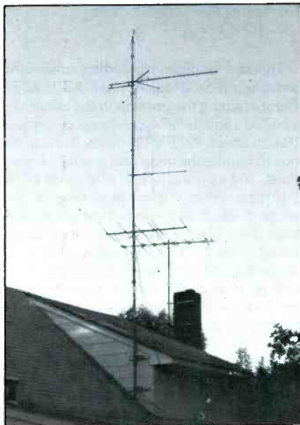
This high-rise antenna farm features from top: a wideband discone, a UHF beam, a 2-meter ham antenna, and a standard FM antenna.
