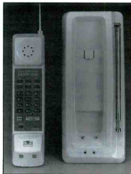
Radio Shack's DuoFone ET-475 is the type of cordless phone found in most homes and offices. It offers four channels in the 46 MHz band.
