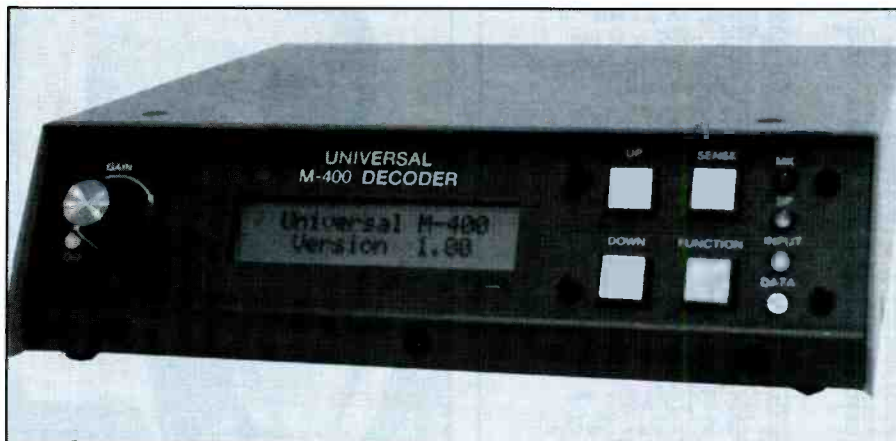
Universal M-400 decoder deciphers messages to and from commercial aircraft in flight.
