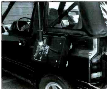
High frequency antenna coupler and whip on a Department of Forestry fire vehicle.
