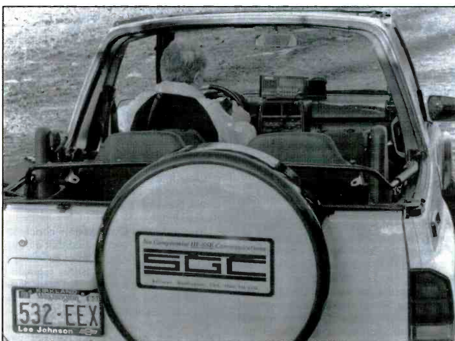
The SGC high frequency SSB remote head up at eye level in the lifeguard jeep.
