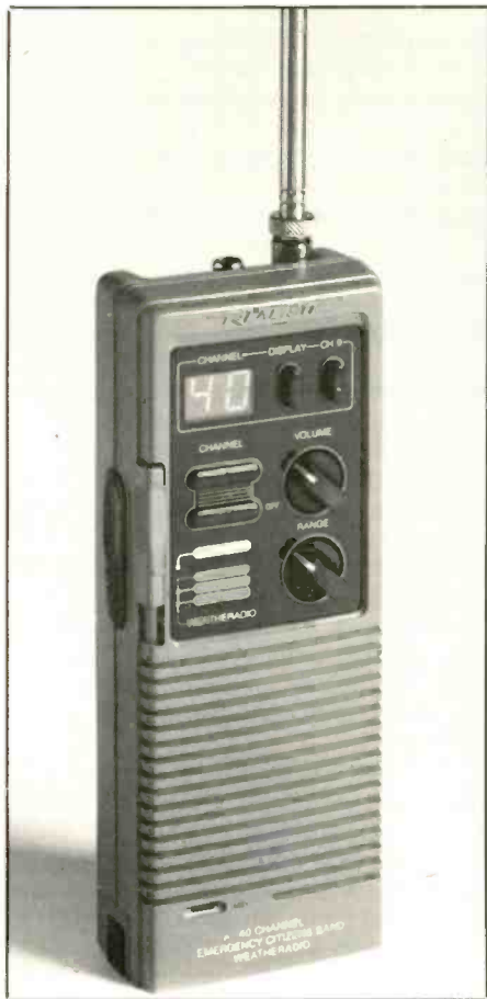
Realistic's TRC-475, from Radio Shack, is an emergency rig intended to be carried in your car and put into service only in time of need. It also receives the 162 MHz NOAA weather broadcasts.
