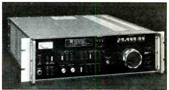
The Watkins-Johnson WH-8718A receiver can tune down to 5 kHz. It's made in Gaithersburg, Maryland.
