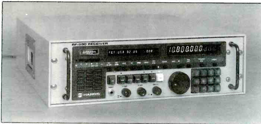
This commercial receiver is the Harris RF-590. It operates from 10 kHz. It's from the Harris Corporation, Rochester, New York.
