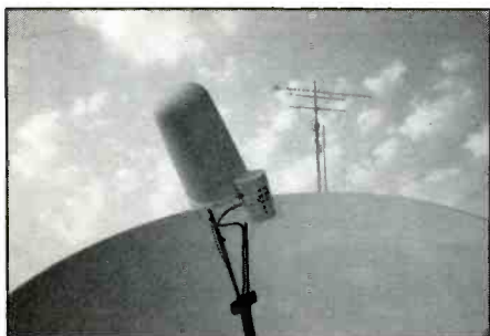
A 1,691 MHz feed horn added to a Satellite TV dish.
