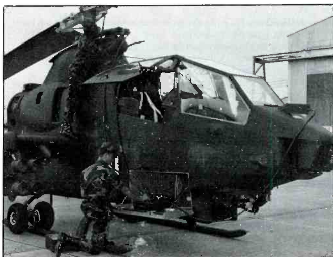
Checking out the AN/ALQ-136(V)1 countermeasures set on an Army AH-1S helo. (U.S. Army photo.)
