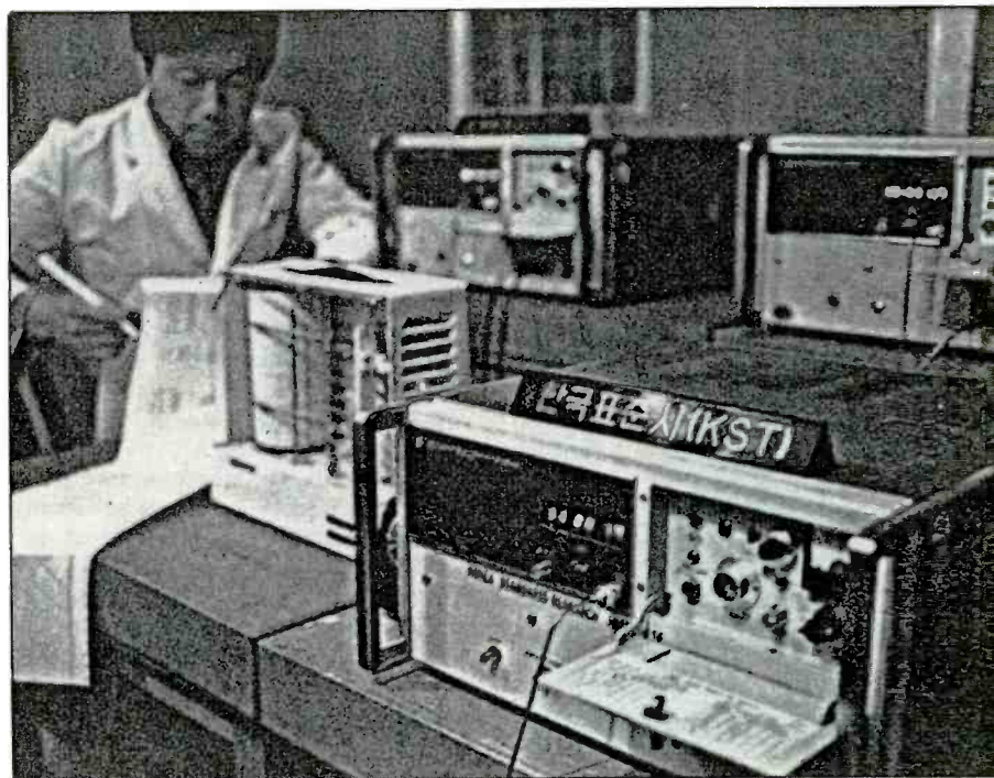
One of the five commercial cesium atomic clocks used to generate the UTC signal broadcast by HLA.
