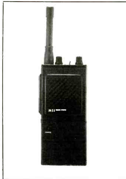
Maxon's GMRS-21 handheld operates in the 460 MHz version of the CB band.
