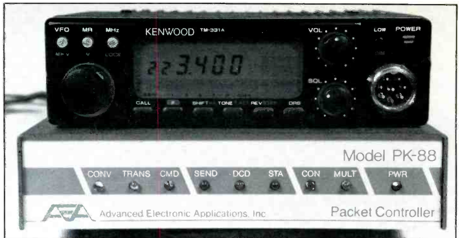
A typical packet station: A VHF-FM transceiver and a terminal-node-controller, or TNC. You supply the personal computer and an antenna, and "Wallah!" you're on the air!
