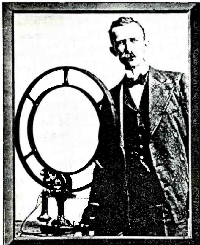
Nathan B. Stubblefield shown posing with his invention around the turn of the century. The loop is apparently the antenna for what may have been an induction-type system.
