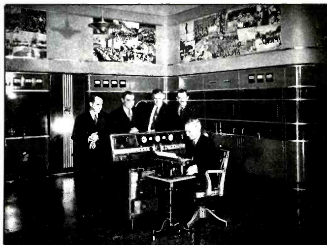
Inside the WLS transmitter building in 1940 showed a 50 kW RCA transmitter attended by a corps of engineers.
