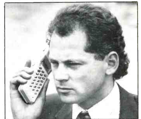
A CT2 handset telephone in use. These short-range services are designed for pedestrian (walk-around) users, rather than mobile subscribers.
