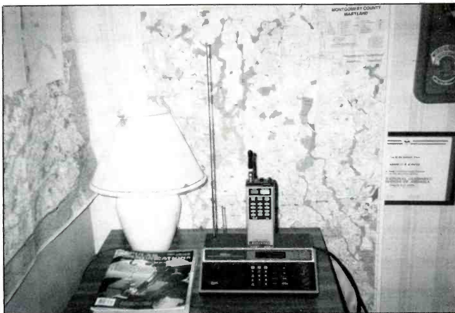
Who says an elaborate listening post is necessary? This more-than-adequate station is owned by Ken Fowler of Fairfax, Virginia. His gear consists of a Uniden Bearcat 800XLT, a Radio Shack PRO-38 and a Radio Shack disccone antenna on the roof.
