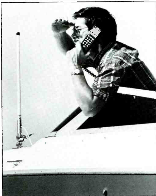
The Shakespeare 4801 fiberglass antenna is suited for marine use.
