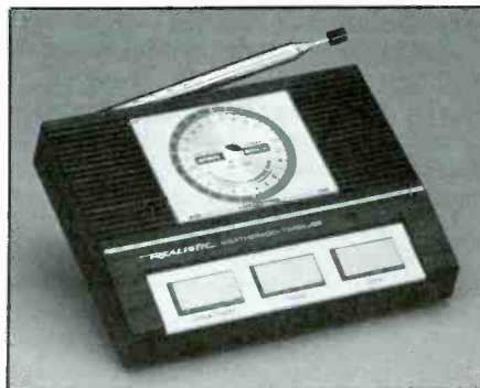
Radio Shack offers this inexpensive WWV receiver to give you reception on three frequencies. It also has the 162 MHz NOAA channels. Sells for less than $40.
