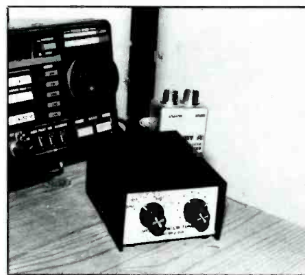
Fig. 3. MFJ-956 SW, MW, and LW tuner.
