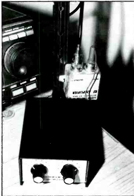
Fig. 5. Tuner and untuned pre-amp in circuit.
