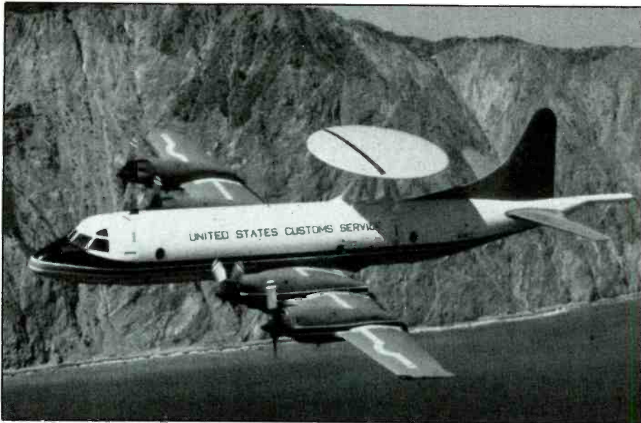
Here is one of the Customs Service's Lockheed P-3 patrol aircraft. The disc on top of the fuselage houses a radar antenna that covers 196,250 square miles in one sweep.
